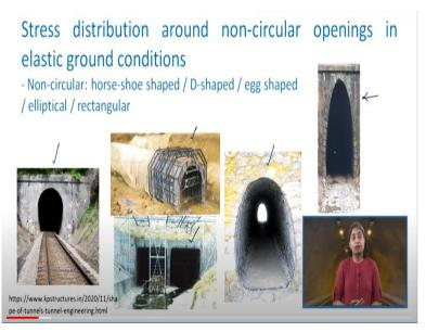
In this slide, I have pasted a few pictures of non-circular tunnels. So, the first picture gives you the idea about the horseshoe-shaped tunnel. You can see why it is called this. Because of the shape of the tunnel, the cross-section of the tunnel is the shape of a horseshoe. Then take a look at this figure this looks like the shape D. So, this is called a D-shaped tunnel. This is an egg-
