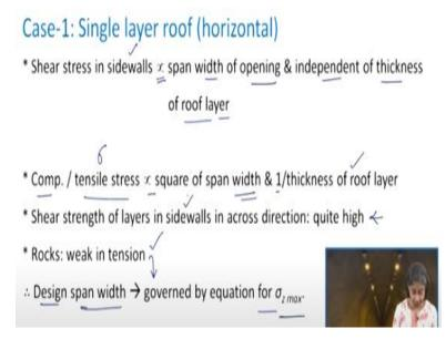
So, if we just try, to take a look here, that the shear stress in the side walls is proportional to the span width of the opening, and it is independent of the thickness of the roof layer. And, the compressive or the tensile stress, which is the  $\sigma$  value, that is the, that is proportional to the square of the span width and inversely proportional to thickness of the roof layer.
