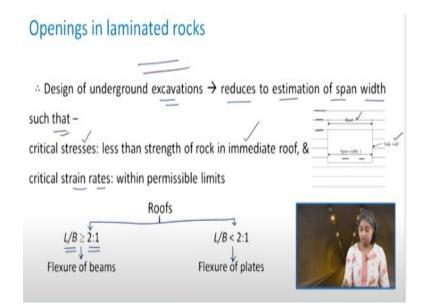
So, the design of underground excavations in the laminated rocks, it reduces to the estimation of span width. Such that critical stresses, they are less than the strength of the rock in the immediate roof, and also the critical strain rates, they are within the permissible limits. See here, I have shown you an excavation which has the span width of l, and the length of the opening which is in the direction perpendicular to the plane of screen, that I am representing as B.
