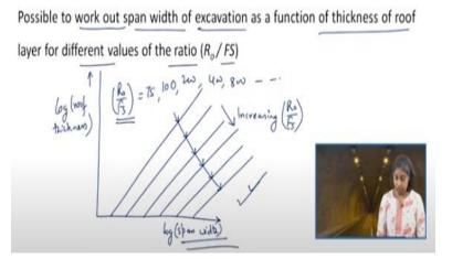
So, what we do is, we work out the span width of the excavation, as a function of thickness of roof for different values of this ratio  $\frac{R_0}{F_s}$ . And, how do we plot it see we take here as log of span width on x axis, and on y axis, we take log of roof thickness, and then we get this kind of set of lines. So, in this direction it is increasing value of r naught upon fs. So, maybe you can have this  $\frac{R_0}{F_s}$  you can have maybe 75, 100, say 200, 400, 800, and so on.
