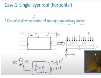
So, we take few cases, so to start with we take the most, simple case that is, when you have the single layer roof, and it is horizontal. So, you see that how it looks like, how the geometry looks like, we have this as the excavation, this is the side wall, and this is the roof, and there is only one layer here, single layer and it has a thickness t. Now, this represents the case of the shallow excavation, and this situation can be there in case of the underground military bunker.
