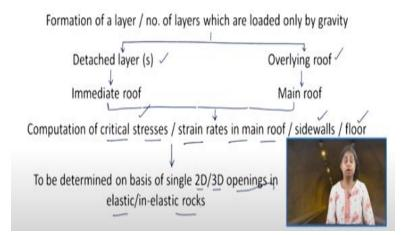
Now, what we have is the formation of a layer or there can be number of layers, which are loaded only by gravity. Now, there is going to be 2 situations, we can have the detached layers or we can have the overlying roof. Further, this detached layer is called as the immediate roof, and overlying roof is called as main roof. I explained you that, what exactly do we mean by detached layer and the overlying roof.
