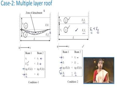
Now, here is a figure with the help of which, I will try to explain to you that, there can be the occurrence of 2 conditions in the case of 2 beams. Please remember that, I will always mark the lower beam as the first beam, which is represented by this number 1, and the upper beam would be given as beam number 2. And, corresponding to beams 1 and 2, you will have the thickness as  $t_1$  and  $t_2$  respectively and flexural rigidity as  $E_1I_1$ , and  $E_2I_2$  respectively.
