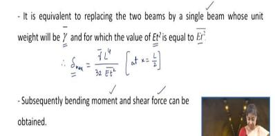
Now, what does this mean I have this  $\overline{\gamma}$  as the average unit weight of 2 beams, or I can write it as  $\overline{\gamma} = \frac{\gamma_1 t_1 + \gamma_2 t_2}{(t_1 + t_2)}$
