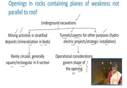
Now, coming to the opening which have the planes of weakness which are not parallel to roof. So, we can have the underground excavation divided into 2 parts or 2 categories. I should say the first one corresponds to the mining activities in stratified deposits. There can be
