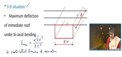
So let us try to take a look that the cases of caverns where you have W by B or L by B is less than or equal to 2 is to 1. We all know that B is the dimension perpendicular to the plane of the screen, and W is the width of the opening. So, in case if the aspect ratio is such that W by B is less than or equal to 2 is to 1, which is in case of caverns. In that case, the immediate roof acts as the rectangular plate which is subjected to biaxial bending.
