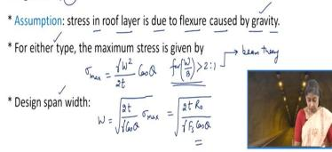
Now, each type of roof, whether it is type 1 or type 2 the angle that is measured between roof and the horizontal we are designating it by theta, and the assumption that is involved here is that the stress in the roof layer is due to the flexure which is caused by gravity. There are no external forces except for the force by gravity. So, for either type of the situation, the maximum stress is given by:
