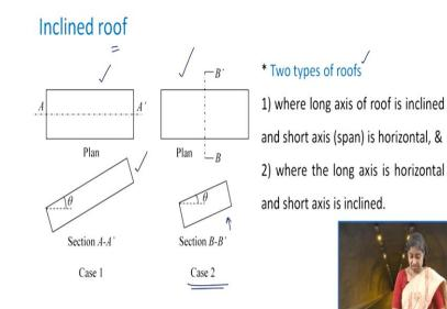
Now as of now, we have discussed only the horizontal layers as a part of roof. But then there can always be the occurrence of the inclined roof. So let us take a look how can we handle such situations. There can be 2 types of roofs. Where we can have 2 situations: first is that the long axis, if the roof is inclined and short axis is horizontal. So, take a look let us see if this long axis and this is what is the short axis.
