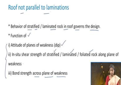
So, how to handle such situation so in this case, the behavior of these stratified or laminated rock in roof governs the design, and it is the function of attitude of the planes of weakness or also called as the dip. Then the in-situ shear strength of the stratified or laminated or foliated rock along the plane of weakness is another governing factor plus the bond strength across the plane of weakness.
