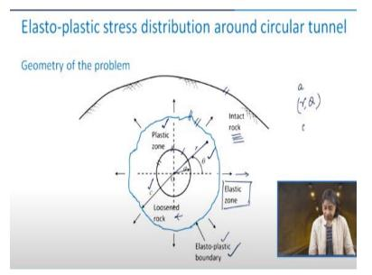
So, first coming to the geometry of the problem, so, here you see that we have the ground surface and this is assumed to be an intact rock. Which is not the situation in the field, in the field what you get is, the rock mass but then to start with we are making this assumption that the excavation is made in intact rock.
