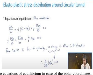
So, let us write the equations of equilibrium in case of the polar coordinates, so, we use the polar coordinate system here. So, what we are going to have is
