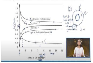
Elasto-plastic stress distribution around circular tunnel
