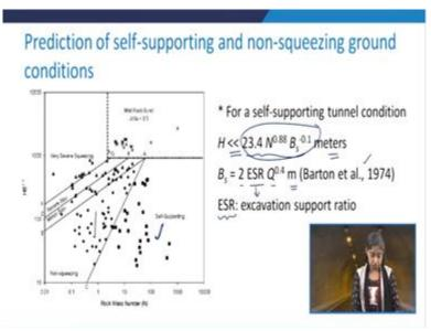
So, this figure we discussed in the previous class, and we saw how this line BA was clearly identifying the two areas, one being the non-squeezing and another being the squeezing ground condition. So, we continue with this, and we try to see some other types of the ground conditions, such as self-supporting and non-squeezing. And also, in the squeezing ground conditions, it has further been classified as minor squeezing, severe squeezing, and very severe squeezing.
