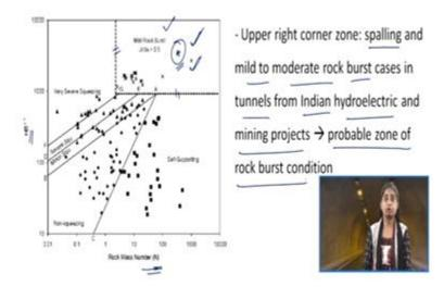
Focus on the rock burst condition because we discussed what is the degree of squeezing? Various degrees of squeezing are based upon the tunnel closure. Now, we focus on the rock burst. So, take a look here at the upper right corner zone, which is shown by this dotted rectangle. This is what is the mild rock burst zone? Here, in this case, if the point corresponding to rock mass number and H into B to the power of 0.1 falls in this zone.
