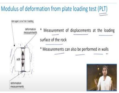
Now, let us take the first in-situ test for the determination of modulus of deformation this is called as plate load test. So, here what we do is in the rock mass, we prepare an edit and there we apply or we put the plates on both the ends and then we apply the load onto these plates and then we measure the deformations. So, this is how we carry out the plate load test, so, this is the measurement of the displacement at the loading surface of the rock.
