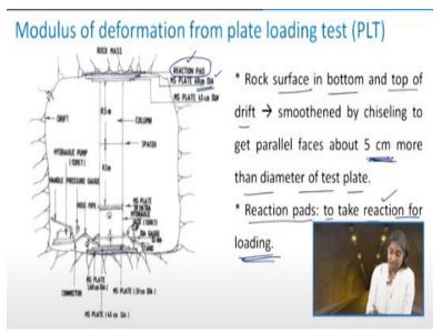
Let us take a look at the test setup, and this will make things clear to you. We use the rock surface in a drift so you see that this is the drift that is prepared. So, the rock surface in the bottom and top of the drift that means here this is what it is the rock surface this is smoothened by chiseling to get the more or less parallel faces about 5 centimeters or more than the diameter of the test plate.
