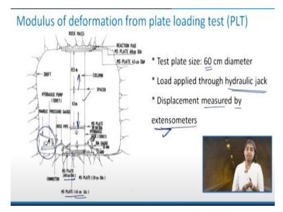
So, the test plate size of 60-centimeter diameter is used so you can see here that, 60-centimeter plate is there which is in contact with the reaction pad. And on top of that, we put another plate which is 45-centimeter diameter, and then somewhere in between we have these spacers. And, with the help of this hydraulic pump here, that is shown we apply the load that is being mobilized and it tries to push the plates in this direction.
