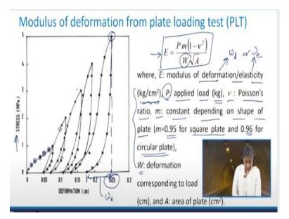
So, what we do is that we apply the load then we wait for some time the deformation to take place, then we remove that load in the stages it is exactly the same as you conduct cyclic plate load test in case of the soils. So, you see various points they tell you that, ok this was the load increment and the corresponding deformation. And, while unloading also it is done in steps not that immediately whole of the load was removed.
