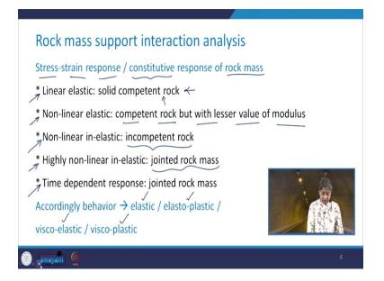
Now, before I go further, let us try to understand first the behaviour of the rock mass and then behaviour of the support system. Then we will try to understand their interaction phenomena. So, as far as the rock mass is concerned, it is material behaviour will be given by stress-strain response or we can call these as constitutive response of the rock mass. Any rock mass can behave in the linear, elastic manner, which is a particular case of the solid competent rock.
