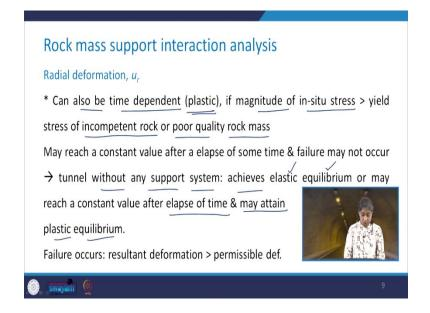
In that case, the radial deformation can also be time-dependent but plastic. So, this is the condition when magnitude of in-situ stress is greater than the yield stress of incompetent, rock or poorquality rock mass. Then it may reach a constant value after some time, and failure may not occur. So, the tunnel without any support system it achieves the elastic equilibrium or it may reach a constant value after elapse of time and may attain the plastic equilibrium.
