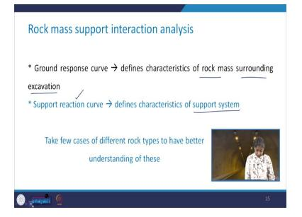
Now, the ground response curve is a term that clearly defines the characteristic of the rock mass surrounding the excavation. So, we have seen that when we talk about rock mass support, interaction or the rock mass tunnel support system, then in that case, we have two components one is the tunnel or the excavation itself, and the other component is the support system.
