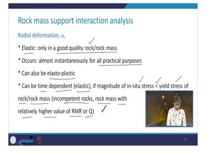
Coming to this radial deformation, it is elastic only in very good quality rock or rock mass. It occurs almost instantaneously for all the practical purposes in case if you have very good quality, rock or rock mass. Then this radial deformation can also be elasto-plastic. It can be time-dependent but elastic if the magnitude of in-situ stress is less than yield stress of rock or rock mass.
