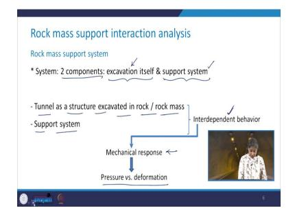
Now, let us combine the two-rock mass, as well as the support system. So, this complete system has two components, as we have seen that it is excavation itself and the support system. Now, depending upon what type of rock mass it is your excavation will show respective material behaviour. Similarly, what type of the support system is needed? Correspondingly, you will have the mechanical behaviour of the support system.
