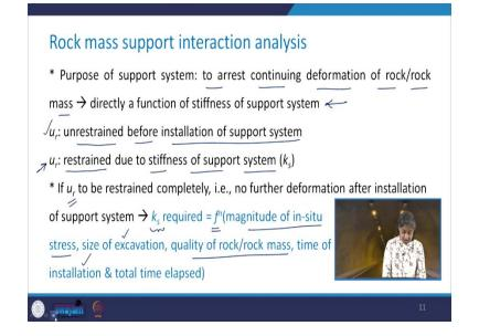
What is the purpose of the support system? This is to arrest the continuing deformation of rock or rock mass, and therefore, it becomes directly a function of stiffness of support system. So, the radial deformation is unrestrained before the installation of the support system. But then, this radial deformation becomes restrained due to the stiffness of the support system after it has been installed.
