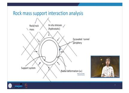
Take a look here. This is the excavation which is done maybe through rock or rock mass. The insitu stresses are considered to be hydrostatic, so, since it is hydrostatic, you see in all the direction it is acting, and the magnitude remains the same. This is what is the excavated tunnel boundary. And then you allow some radial deformation to take place. So, this is how the radial deformation  $u_r$  will be measured?
