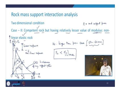
Let us take the next case of the competent rock, but it has relatively lesser value of modulus, and the behaviour is non-linear elastic rock. So, how does this look like the behaviour? Let us take a look here so, again on x-axis, we have the radial deformation, and on y-axis, we have the radial support pressure, say here. Of course, you have P<sub>i</sub> and here this is where you want it to be completely arrested all the deformations, it is 0.
