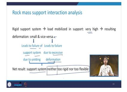
So, in case, if the resulting deformations are extremely small, these lead to the failure of support system due to yielding of the supports, but in case of the other one that is when you have very low load which is mobilized in the support and the resulting deformations are very high. In that case, the failure is due to the excessive deformation. So, the net result basically is the support system which is neither too rigid nor too flexible.
