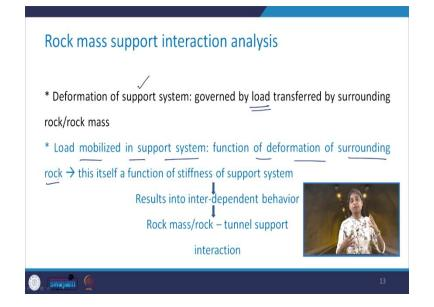
So, basically, the deformation will be governed by what is the load that is being transferred by the surrounding rock or rock mass. So, the load that is mobilized in the support system becomes the function of deformation of the surrounding rock, which itself is a function of stiffness of the support system. So, you see what exactly is happening here? That the stiffness of the support system is a function of deformation, and deformation is a function of the support system.
