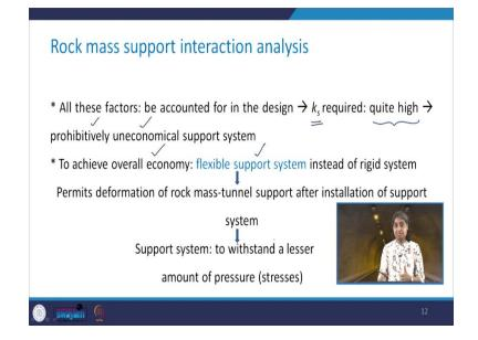
So, when we go for the design of the support system, all these factors should be accounted for. So, if you want to restrain the complete deformation, the required stiffness of the support system, which we are representing as case is going to be quite high. And this will make the support system prohibitively uneconomical. So, to achieve the overall economy, one should go for the flexible support system instead of a rigid system.
