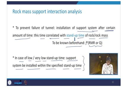
What should we do to prevent the failure of the tunnel? We should install the support system after certain amount of time. Now, why we should install the system after certain amount of time? Because if we apply the system immediately, there is going to be lot of support pressure on to the support system, and we need to go for extremely rigid support system and that may not be economical.
