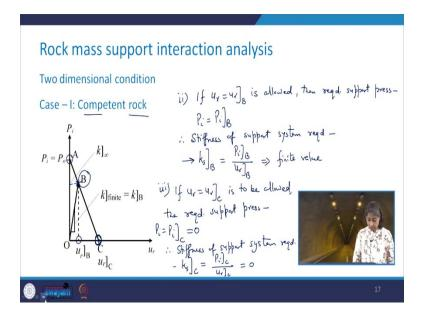
Then I take the other case that is the second one now, if  $u_r = u_r$  at B means here this point. So, if this is allowed then the required support pressure. What it is going to be? It will be  $P_i$  will be equal to  $P_i$  at point B so, you see that here. So, what will be the stiffness of the support system in this case? Which is required is going to be case at point B will be equal to:
