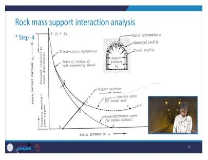
And therefore, the support reaction curve, it now becomes this DEF line. So, this is what is your support reaction curve.
