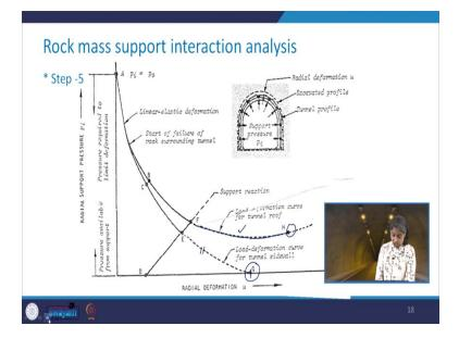
So, you see here that this portion in the side wall this becomes equal to zero. Here, the support pressure is zero in this case. But what will happen to roof? So, on the other hand, the support which is required to limit the deformation of roof it first drops to a minimum and then again it becomes or it begins to increase. Take a look here, first it reduces little bit and then it goes and increases to this point H.
