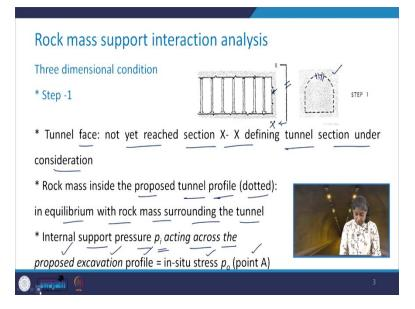
So, we take the first step where the section x-x is a head of the tunnel face here. So, you will see only the rock mass if you cut at section x-x you will see only the rock mass but of course, since the tunnel is being driven and therefore, we are showing this as a dotted line. So, basically tunnel face has not yet reached section x-x, defining the tunnel section under consideration.
