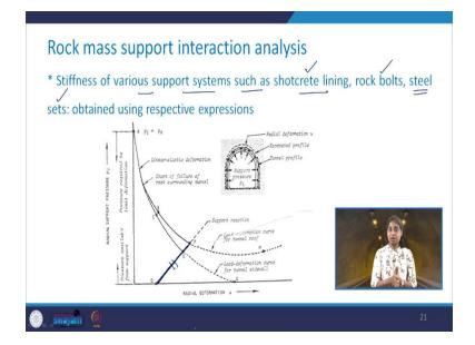
So, this is how with reference to a 3-dimensional situation, you can visualize that how the support reaction curve and ground response curve one can develop. Now, coming to the stiffness of the various support systems which can be shotcrete lining, rock bolts, steel sets. These can be obtained using respective expressions. This we will learn when we discuss about the Ladani's rock mass support interaction analysis.
