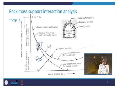
So, therefore, we are going to have two ground response curves, one will be for the tunnel roof, and another will be for the side walls. So, corresponding to that, here is the point B that we were talking about, and this is in the roof portion, and the corresponding point in the side wall is going to be the point C here.
