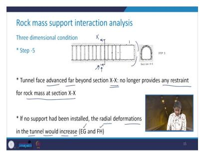
Now, we come to the step-5. So, you see how with respect to every step? We are trying to draw the ground response curve, as well as the support reaction curve. Now, we go to the next step, which is the step-5. So, what I am going to do in this case? That the tunnel face is advanced far beyond this section x-x, you see. Okay, where there is no restraint for the rock mass at x-x section. You see, there is no restraint from this rock mass because it is much far.
