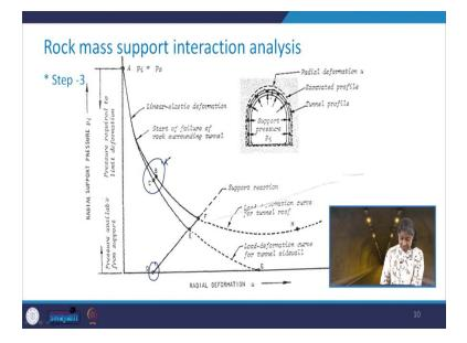
So, you see that this is the point D because now the support system is coming into picture. So, simultaneously now, we will be starting drawing the support reaction curve along with the ground response, and since this deformation is not there right now at point D. So, basically, B and C will be the same ground response curve or the same points at ground response curve in the step-3 as well.
