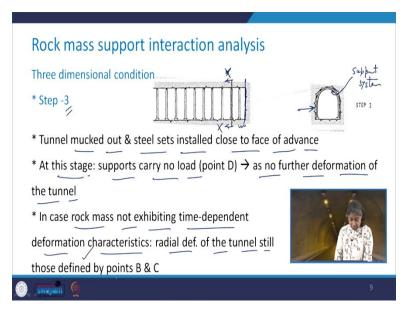
Coming to the third step, what we do? We advance the tunnel up to this in the previous step, but we did not provide the support up to section x-x, which is here. So now, what we are going to do is? We have provided in this step the support, which is beyond section x-x, so you see in the cross-section, you will see the excavated surface and also the support system. So, what is the step-3? That tunnel was marked out, and steel sets were installed close to the face of advance.
