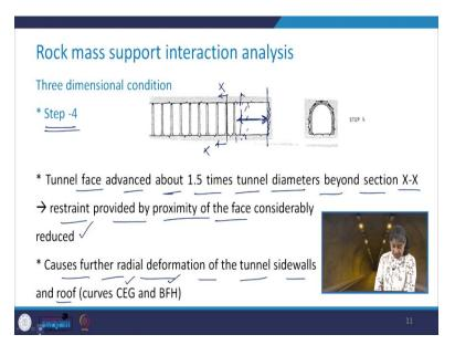
Coming to the fourth situation, what will happen now? So, we have installed the support system and further advanced the tunnel that means now tunnel face has gone beyond the section x-x, and the it is not that the support system has been installed up to the face of the tunnel. So, tunnel face
