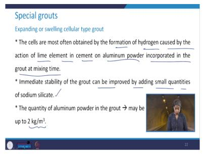
The cells are most often obtained by the formation of hydrogen, which is caused by the action of lime element in cement on aluminum powder incorporated in the grout at the mixing time. The immediate stability of the grout can be improved by adding some small quantities of sodium silicate and the quantity of the aluminum powder in the grout it can be maybe up to 2 kg per meter cube.
