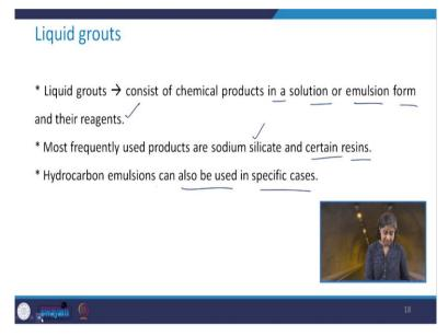
Coming to the liquid grouts. These consist of chemical products in a solution or emulsion form and their reagents. Most frequently used products are sodium silicate, and some resins, hydrocarbon emulsions can also be used in some of the cases as the part of the liquid grout. (Refer Slide Time: 18:23)
