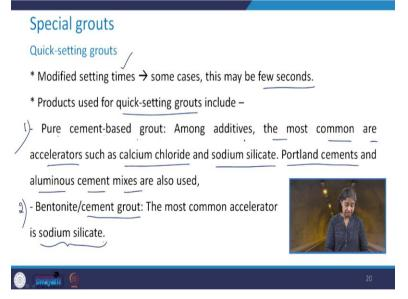
So, let us take a look about the quick setting grouts. So, here these have the modified setting times. In some cases, these maybe few seconds. The products which are used for quick setting grouts these include the number one is pure cement-based grout. So, among additives the most common are accelerators such as calcium chloride and sodium silicate. In this cases, portland cements and aluminous cement mixes are also used.
