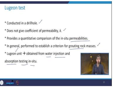
Coming to some aspects related to this test, I will not be discussing in detail, but we will try to give you an overall idea, what this test is all about. So, basically this is conducted in a drill hole it really does not give us the coefficient of permeability. However, it provides a quantitative comparison of the in-situ permeabilities. So, in general these test are performed to establish a criterion for grouting the rock masses.
