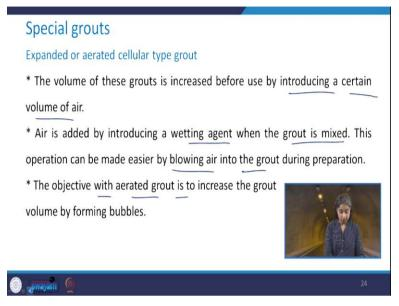
The volume of these grouts is increased before the use by introducing a certain amount of air, certain volume of air. The air is added by introducing a wetting agent when the grout is mixed. So, this operation can be made easier by blowing air into the grout during its preparation itself. So, the objective with the aerated grout is to increase the grout volume by forming the bubbles into it.
