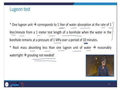
So, what do we mean by one lugeon unit? See, this is a bit long definition, but focus and then, you will realize that, it is very easy to follow. So, one lugeon unit corresponds to one liter of water absorption at a rate of 1 liter per minute from a 1-meter test length of the borehole, when the water in the borehole remains at a pressure of 1 megapascal over a period of 10 minutes.
