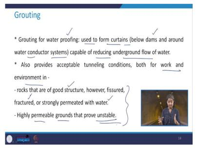
Grouting is done for the water proofing as well. Here it used to form curtains especially below the dams and, around the water conductor systems and these curtains, they are capable of reducing the underground flow of water. This also provides acceptable tunneling conditions both for work and the environment in the rocks which are of good structure, but they are fissured, fractured, or strongly permeated with water and, these are also helpful in highly permeable ground that prove to be unstable.
