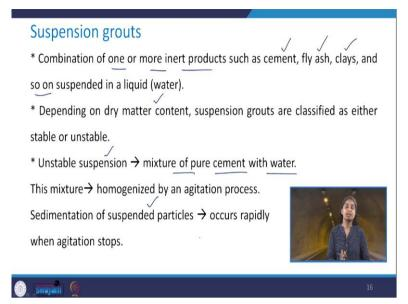
So, let us take a look on the suspension type of grouts. So, it is the combination of one or more inert products such as cement, fly ash, clays and so on which are suspended in the liquid which is water. Now, depending upon the dry matter content suspension grouts are classified as either, stable or unstable. So, when we talk about the unstable suspension this means that, it is the mixture of pure cement with water.
