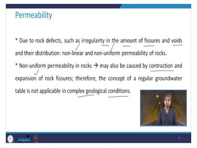
Now, due to these rock defects such as irregularity in the amount of fissures and voids and their distribution, permeability of the rocks are non-linear and non-uniform. So, this non-uniform permeability in rocks, these may also be caused by the contraction and expansion of rock fissures and therefore the concept of a regular groundwater table is typically not applicable in the complex geological conditions.
