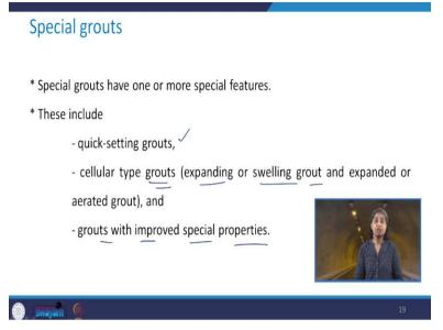
Now, coming to some of the special grouts. So, here these have one or more special features such as quick setting grouts then we have the cellular type grouts. So, what happens in this case these are expanding, or swelling grout, and expanded or aerated grout, and the third one is the grouts with improved special properties.
