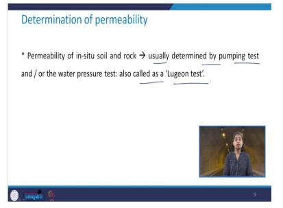
So, the permeability of in-situ soil and rock, these are usually determined by the pumping test and or the water pressure test which is also called as the lugeon test.
