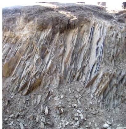
Meta-siltstones of Hasthoji formation: thinly foliated & excessive weathering close to surface
