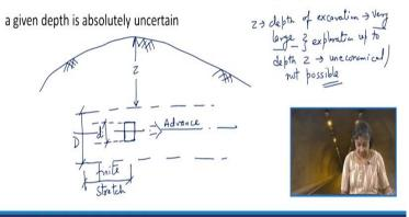
Now the next type of the underground excavation it includes the now the next type of underground excavations includes the pilot tunnel. Now, this is essential to excavate in situations where prediction of geological conditions at a given depth is absolutely uncertain. So, before we go for the main tunnel, we have to construct the pilot tunnel. Let us see how it looks like, so this is what is your ground condition and say this is the centre line for the tunnel.
