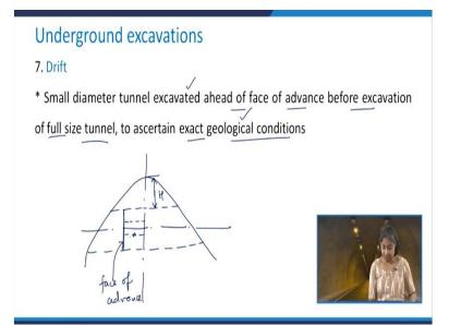
Now, the next structure is called as drift. It is the small diameter tunnel which is excavated ahead of phase of advance before the excavation of a full-size tunnel to ascertain the exact geological conditions. You know that these rocks and rock masses they are naturally occurring material and lot of uncertainties are involved which may not be clear during the exploration program. So sometimes, you get a few surprises when you go for the tunnelling.
