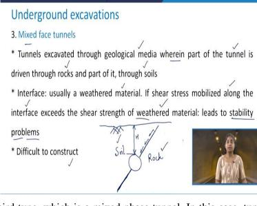
Coming to the third type, which is a mixed phase tunnel. In this case, tunnels are excavated through geological media wherein part of the tunnel is driven through rocks and part of it through soils. That is why it is called mixed face tunnels, so the interface is usually a
