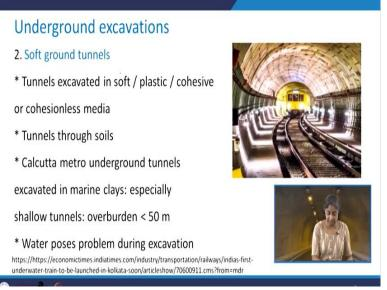
Then the second category includes soft ground tunnels. These tunnels are excavated in soft plastic cohesive or cohesion-less media basically tunnels through soils. They fall under this category. An example of such a tunnel is Calcutta metro underground tunnel which is excavated in marine clays. These are especially shallow tunnels with an overburden of less than 50 meters.
