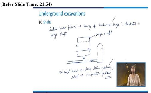
Then these shafts can also be used in for the surge tanks; let us see how they work. So in case if there is the sudden power failure, then what happens is that the energy of the backward surge is dissipated in surge shafts. Let us see how with the help of a figure, we can see this. So there is this surge shaft, so let us say the earlier the water table was here in this level of the water. And in case of the sudden power failure, this water level goes up, and it may be like this here.
