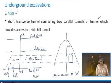
So, the next type of underground excavation it includes adits. So, these are short transverse tunnel which connects to 2 parallel tunnels. These are the tunnels that provide access to a side hill tunnel so let us look with the help of a figure that is how it looks. So here, I will draw the plan as well as the cross-section to give you the idea. So let us say that here this is what is the foot of the hill. And I take a section which is say it is AA.
