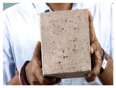
So, this is a cubicle sample you can see for a concrete mix.
