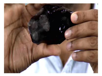
We also have bitumen. So, this is mostly I mean now, it is more of semi solid in nature, because the temperature of the room is around 25 to 26 degrees Celsius, but if you heat it, this will become fluid and if you cool it down, it will become solid in nature. So, this is more of a viscoelastic material. And we will be discussing about this material in detail in our lecture series.
