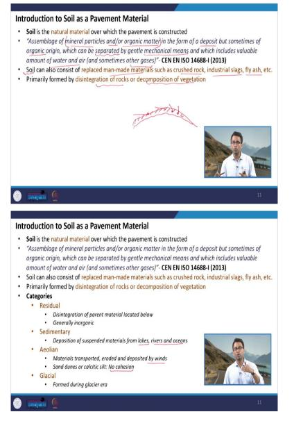
So, soil can be defined as a natural material over which the pavement is constructed. So, this is the simple definition of soil considering that we are going to use it in pavement construction. So, if you see the definition given in CEN EN ISO 14688. The definition states that soil is an assemblage of mineral particles. Now, these are some critical words which tells us, which gives us much indication about the properties of soil.
