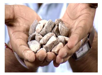
We also have aggregates here as I mentioned that this is used for the construction of granular layer this is used for the production of bituminous mixtures, concrete mixtures and so on. So, these are some aggregates in my hand, though these are single sized aggregates, which I am showing you presently, but in practice in a particular layer, the aggregates can be present in various different sizes depending on the target gradation, we are going to talk about these aspects as we move forward.
