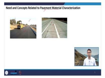
So, when you see the term pavement material, we have a predominant term here is pavement. So, we are learning about materials that are used in pavement. So, just to begin just to have a feel about this subject, let us try to see the two basic pavements that are typically used in construction. So, we have a flexible pavement here and we have a rigid pavement here. So, these are the general terminologies.
