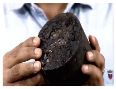
Then we have a bituminous mixture here. So, this mixture is something which you can see in the picture here. So, this is the bituminous mixture composed of aggregates of different sizes and bitumen mixed together and we also have some quantity of air voids within the volume.
