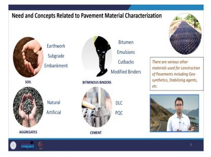
So, some of the basic materials that are used in construction, it includes soil, it includes bituminous binders, aggregates, cement, and there are various other materials, but these are some of the very primary materials that are used in construction. For example, soil is used in the construction in earthwork, in subgrade, in embankment.
