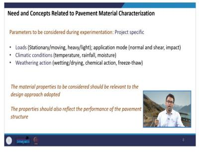
So, some of the critical parameters which I have to consider before doing the experimentation is load, load is one of the very important parameter. So, I have to understand that the material which I am going to use will be subjected to or the material which I am going to use in the pavement system. So, that pavement system will be subjected to which type of load.
