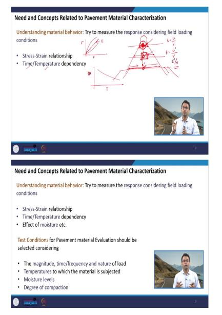
As I have been mentioning continuously that we have to measure the response considering the field loading conditions. And the responses can be seen in various different ways. For example, I can plot a stress strain relationship while doing the testing of the material. So that will, for example, if I am looking at the elastic modulus, then the stress strain property will give me the modulus.
