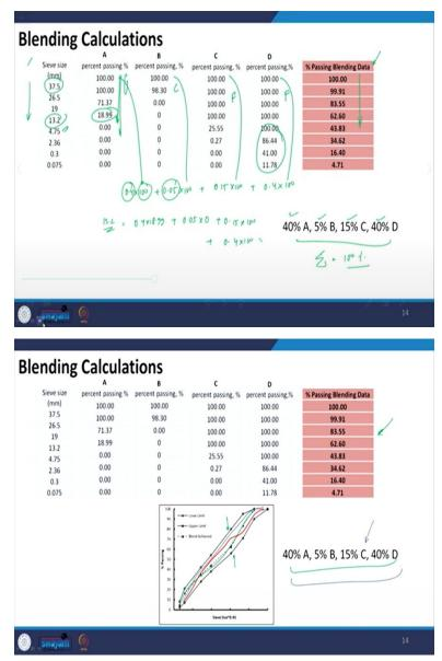
Let us say you have these standard sieves here I have taken another gradation having a different set of sieves here ranging from 37.5 to 75 micron. Let us say you have the first stock pile and you did the sieve size analysis of the stockpile you calculated the percentage passing corresponding to different sieve sizes and you got these values.
