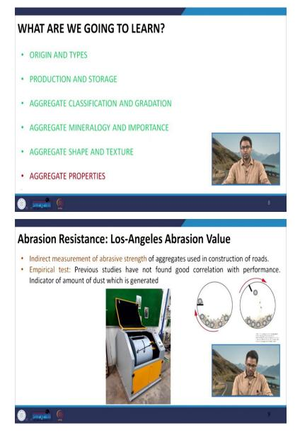
So, let us start discussing about other tests today, which are further used to quantify different other characteristics of the mineral aggregates that we use in pavement construction. Today, we will start with the Los Angeles Abrasion Value test, which is used to know about the resistance of the aggregates to abrasive forces.
