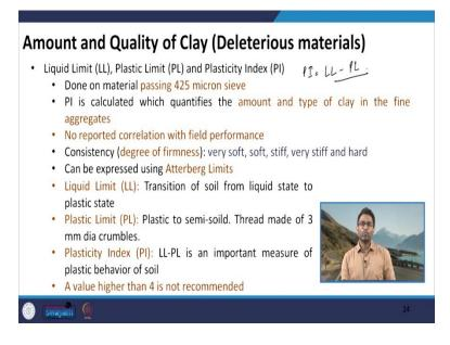
Well, we have other simple tests that are generally used in the study of soils to quantify the properties of the fine materials such as clay, a set of these tests are related to the Atterberg limits, where we are trying to find out the liquid limit plastic limit and plasticity index, which gives us indication about the plastic properties of the fine materials.
