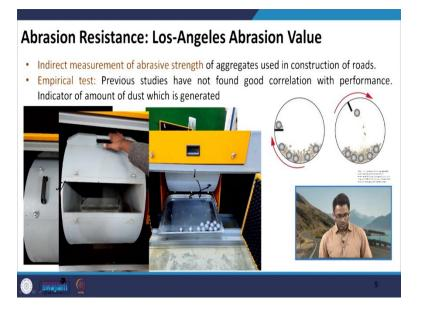
This has an opening here, where the materials and abrasive charges are put this is one picture showing the different charges, I have two charges with me just to have a visual idea of how these charges looks like. So, you can see that these are spherical balls which are used as charges in the Los Angeles Abrasion machine.
