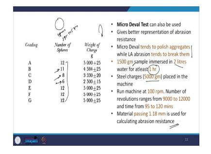
Well, this shows the choice of number of aggregate charges and the corresponding weight. So, actually the diameter of this ball, which we take in Los Angeles Abrasion test is approximately 48 mm. So, this is the dia and the weight somewhere lies between 390 to 445 grams. So, that is the individual weight.
