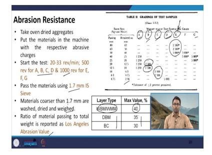
So, talking about the steps of the Los Angeles Abrasion test, first we have to take oven dried aggregates. Now, the type of aggregates which we have to choose the size of aggregate which we have to take, it depends on the type of gradation, I will show you it in a table. So, what we will do after we choose the appropriate material, we will put this material inside the machine with the respective abrasive charges.
