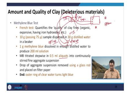
Now, we will discuss about the next test which is not typically used in India, but is a French specification basically. So, this is a French test and in fact a very interesting and good test to quantify the quality of clay fines. So, this will not tell us about specifically about the amount of clay fines but it will say that, that though you have particles of smaller sizes in your mix.
