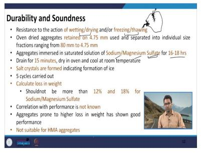
So, specifically in cold weather regions what happens is that, because of this capillary rise of the water, the water can get freeze inside the pores of the aggregates or not only capillary rise the general movement of water and the formation of ice this water can get freeze within the pores of the aggregates.
