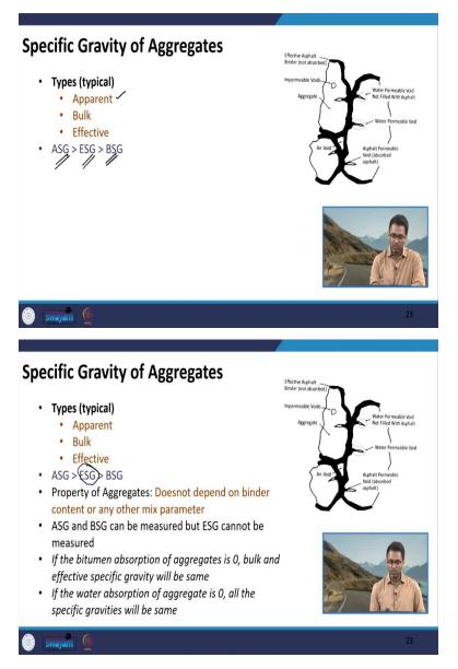
We will talk in detail when we discuss about the mix design, but I hope the concept of apparent, bulk and effective specific gravity is clear to you since the volume of apparent specific gravity is the least here that is why apparent specific gravity is highest followed by effective specific gravity followed by bulk specific gravity.
