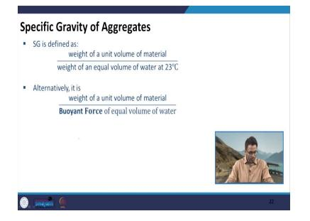
We have also discussed about the properties related to fine aggregates such as amount of clay and the quality of clay by understanding about the sand equivalent value test about we have also looked at the methylene blue value test and also at the Atterberg limits. So, let us continue discussing about the aggregate properties and today we will start with understanding about the specific gravity of the aggregates.
