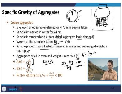
Now, let us talk about the experimental procedure of determining the specific gravity of aggregates in the laboratory, we have different method for coarse aggregate we have different method for fine aggregates. So, let us discuss both what we do for coarse aggregate we will take 5 kg of oven dried sample that is retained on 4.75 mm sieve. It can be of different sizes also greater than 4.75 mm sieve.
