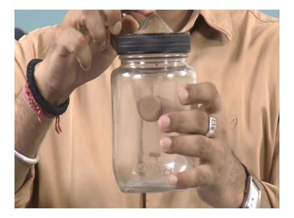
So, the problem actually lies in the determination of the saturated surface dry weight it has been observed that the repeatability of saturated surface drying is not very good. And in fact when we talk about specific gravity, we need accurate results at least up to three significant digits, it becomes critical for correct measurement of specific gravity in the laboratory.
