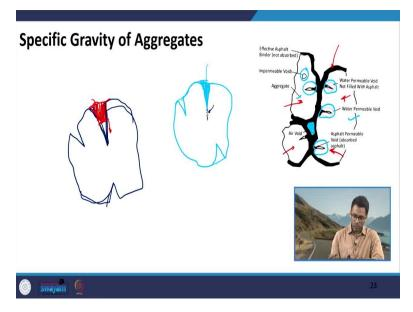
I am taking this example of a bituminous mixture because actually in bituminous mixture, there are different specific gravities which we are interested in this is taken from the Asphalt institute handbook MS2, you can see that there are four aggregates that are shown here from the metrics of the bituminous mixture, then I will try to explain more about this picture.
