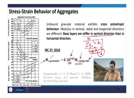
Most of these Studies have shown that granular materials are in fact more complicated in nature, and they so cross an isotropic behavior, which means that the modulus in different directions are also different. Usually, when we talk about pavement construction the base layers or the sub bass layers, they are stiffer in the vertical direction than the horizontal direction.
