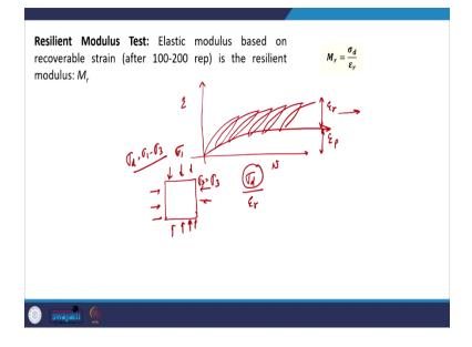
So, resilient modulus is the elastic modulus under repetitive loading, after certain cycles of repetitive loading, what we expect that the material will have no additional permanent strain, whatever permanent strain would have taken place in the initial cycle will remain constant. So, now based on the recoverable strain the amount of recovery which has taken place, we will Define the resilient modulus.
