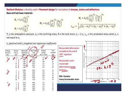
And this is what the Strain gauges have given the result, that when we apply a diabetic stress of one PSI, the recoverable deformation which using the strain gauge we can calculate is 0.264. So, this is in unit of 0.001 inches, this is what the instrument or the equipment give us for the corresponding material, alright.
