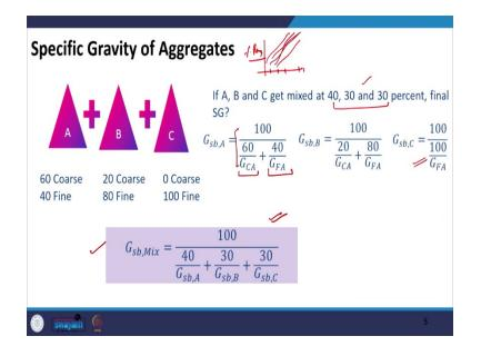
And in stockpile A, we have 60 percent materials which are larger than 4.75 mm sieve and we have 40 percent material which are finer than 4.75 MMC. Similarly, let us say we have a stockpile B with 20 percent coarse Aggregates and 80 percent fine Aggregate and we have a stockpile which is a fine aggregate stockpile.
