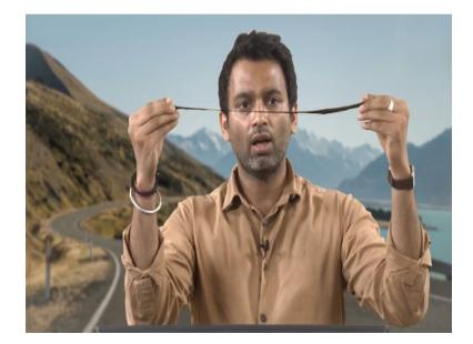
Here if you see I have a small bitumen sample, now this bitumen sample can be shaped now because it is more of you know in a viscoelastic state, so let us see what happens when I start stretching this bitumen sample. So, please note that I am stretching this sample at a very slow rate now, I am applying a force but very slowly from both the sides.
