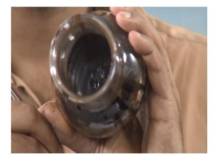
This is a bituminous mix which is produced through impact compaction in the laboratory, this mix which you are seeing it comprises of graded mineral aggregates and bitumen. So, the blackish color which this mix has is basically due to the presence of bitumen, in this mix the aggregate particles are kept together through the binding action of bitumen, I also have brought with me today a jar with some bitumen sample.
