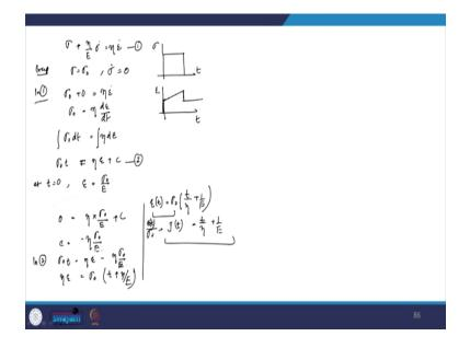
So, our constitutive equation was  $\sigma + \frac{\eta}{E} \times \dot{\sigma} = \eta \dot{\varepsilon}$ . So, when it is a creep experiment sigma is equal to  $\sigma_0$  and  $\dot{\sigma} = 0$  because this is a constant. So, derivative will be equal to 0. Let us say this is equation 1. So, therefore, in equation 1 we can write  $\sigma_0 + 0 = \eta \dot{\varepsilon}$ ,  $\sigma_0 = \eta \frac{d\varepsilon}{dt}$ .
