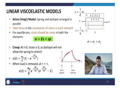
So, therefore, if we go back and try to see what we have just derived, we have the value of epsilon t in the creep loading and when the load is removed at  $t = \tau$ , we have the expression for the strain after that particular point. Here what we see that at t = 0, we have an viscous response.
