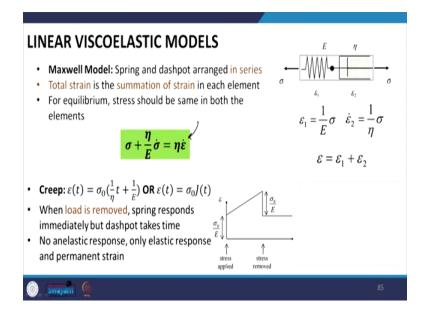
And this is what is shown in this particular figure and this is the response of a Maxwell element when it is subjected to a creep loading. And if you can see in this particular graph that this particular model cannot explain the n elastic response which is typical for a viscoelastic material and only elastic and permanent strain can be explained using this particular model. So, definitely only the Maxwell model cannot be used to describe the response of a viscoelastic material.
