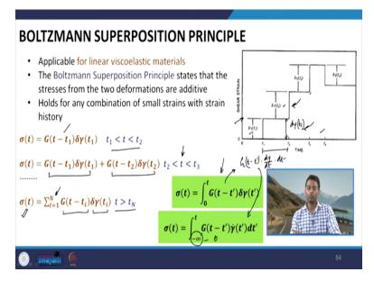
Now, Boltzmann superposition principle is applicable only for linear viscoelastic materials that is viscoelastic materials which are subjected to lower value of strains. So, the Boltzmann superposition principle, it states that the stresses from two deformations or the strain history of the viscoelastic materials are additive in nature. Let us understand this using a step strain experiment.
