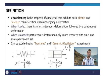
The term viscoelasticity indicates that a material which has such kind of property that is viscoelasticity will exhibit both elastic and viscous response. Now, what do we mean by an elastic and a viscous response? To understand this, let us imagine that we have a spring system which is a representation of an elastic system.
