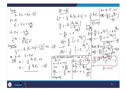
Let us just first write down that the constitutive equation is equal to  $\sigma = E\varepsilon + \eta \dot{\varepsilon}$ . So, in creep experiment  $\sigma = \sigma_0$ . So, therefore, if we put it in equation 1, we get  $\sigma_0 = E\varepsilon + \eta \frac{d\varepsilon}{dt}$ . So, here we can write that  $\sigma_0 - E\varepsilon = \eta \frac{d\varepsilon}{dt}$ .
