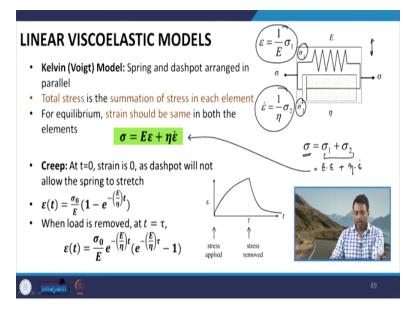
In this model the spring and the dashpot they are arranged in parallel to each other. So, here the total stress is, will be the summation of the stress in each element. So, if we know the stress  $\sigma_1$ , if we know the stress  $\sigma_2$ . So, the total stress  $\sigma = \sigma_1 + \sigma_2$  and the strain in both the elements for equilibrium should be same. So, these are the two conditions in the Kelvin model.
