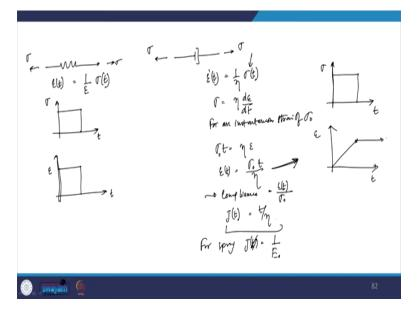
As I mentioned in the first slide that a purely elastic material can be characterized as a spring system. Let us say this is a spring system and we are performing an experiment and we are applying a load or a stress of  $\sigma$ . So, if we try to see the response of the material, this will be equal to  $\frac{1}{F} \times \sigma(t)$ . If we try to see that how the variation will look like.
