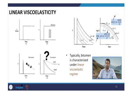
So, this here you can see we are applying a step strain to the material and we are keeping the strain constant after a particular position and we try to see how the response of different materials will be. As I said that a purely Hookean material, it can be represented as a spring element, how it will respond? So, there will be no stress relaxation as such and the stress will be proportional to strain.
