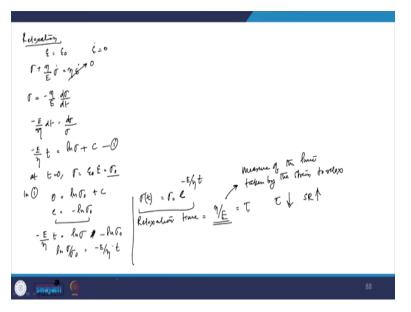
So, in a relaxation experiment, so we are discussing about the Maxwell model here. What we are doing, we are applying a constant strain and we are seeing the stress relaxation. So, if you can recall the constitutive equation was  $\sigma + \frac{\eta}{E} \times \dot{\sigma} = \eta \dot{\varepsilon}$ . So, here  $\dot{\varepsilon} = 0$ . So, this becomes equal to 0. So, we have
