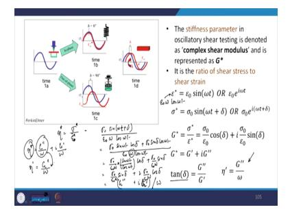
There is another term which is called as the loss tangent or this is the damping component of the material, it describes the damping or the tendency or describes how well the material can absorb or lose energy. So, this is called as loss tangent  $tan\delta$  which is described as the  $tan\delta = \frac{G''}{G'}$ .
