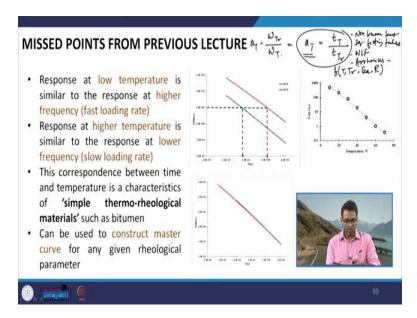
Coming to this particular slide which we discussed regarding the time temperature superposition principle, I explained to you that this principle is applicable for linear viscoelastic material and we discussed that how the response at different temperatures can be superimposed to another reference temperature by multiplying the time with a shift factor.
