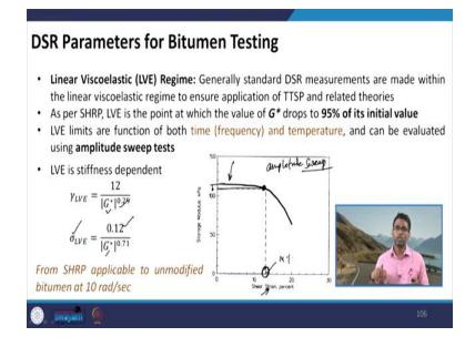
Generally the standard DSR measurements as I said are made within the linear viscoelastic regime. When we are applying time temperature superposition principle, when we are applying several other theories to explain the behavior of the material, these principles and theories necessitates that the material should be within the linear viscoelastic regime. So, therefore, it is important to find out the linear viscoelastic regime. And how do we define it?
