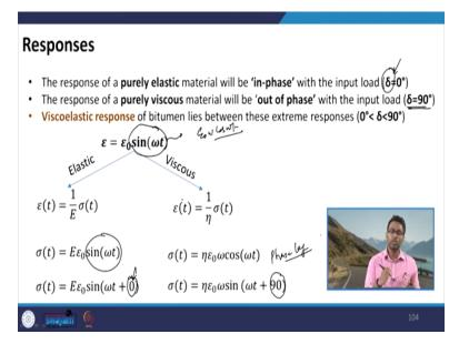
So, now let us move forward and try to understand more about the rheological properties in combination or linking it with the viscoelastic characteristics. So, when we are doing an auxiliary testing you will see that for a purely elastic material. So, let us say we are measuring the properties of a purely elastic material using the DSR the response will be in phase with the input load.
