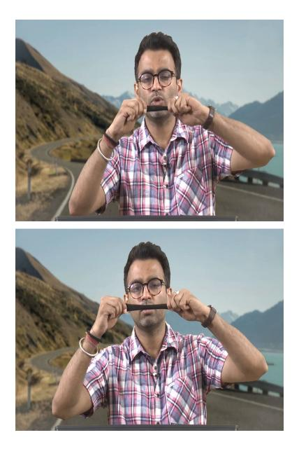
And then what I am trying to do here and just stretching this to some distance, I am just stretching this to some distance, and I am keeping it on the slab. The same I am doing with this I am stretching it almost to the same distance alright. Well I have to apply more pressure because this is a modified bitumen same distance and again I am keeping it on the slab.
