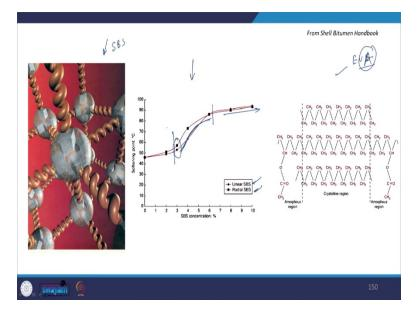
These are some pictures explaining some of the common modifiers for example, this is an animated description of SBS where they show that we have polystyrene blocks and we have a mid-block which is a butadiene segment. Here the polystyrene blocks they impart the toughness to the structure they provide the stiffness to the structure. Whereas, the butadiene segment they provides the more of the rubbery properties to the SBS system.
