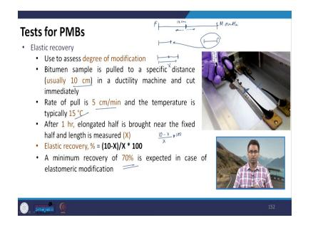
Then we have elastic recovery test. So, this is used to assess the degree of modification. So, here what we do, this is almost like a ductility test which we have discussed previously. So, we have again a briquette here which is filled with bitumen and then we will stretch the briquette at a specific rate and this rate is usually 5 centimeter per minute, but here the test temperature is typically 15 degrees Celsius.
