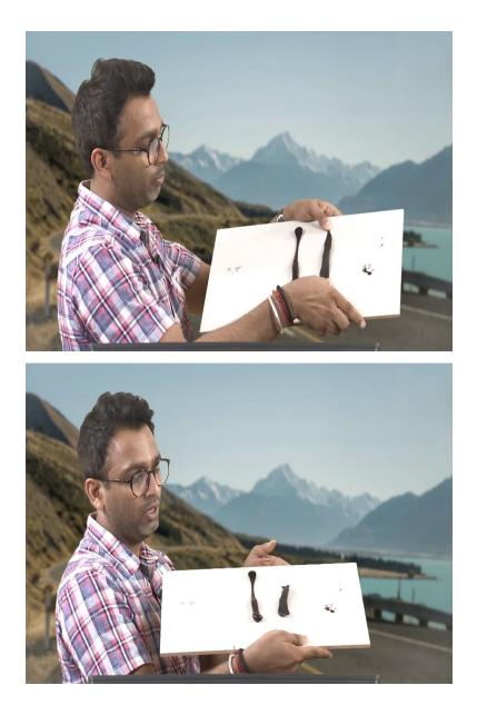
So, you see I am trying to stretch the one which I am not holding is the conventional bitumen and this is the modified bitumen. As soon as I leave this you can see that it tries to contract and it tries to recover. Here, you can see, are initially I stretch to the same length, but now the length is reduced. So, I am trying to keep it here for some time.
