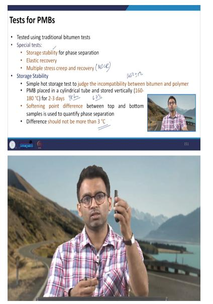
One of the most important tests includes storage stability test, which is done to assess the phase separation. As we have discussed that there can be a tendency that the polymer phase can get separated from the bitumen phase, if the compatibility between the bitumen and the polymer is not proper. So, we want to quantify that and here we can use the storage stability test.
