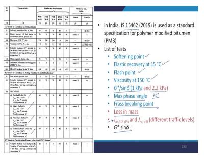
So, this is again a snapshot from IS 15462 which we use in India as a specification for polymer modified bitumen. Most of the test here we have discussed previously and again some of the tests we have discussed today. So, if you see the list of test on unaged condition, we have softening point test, elastic recovery test, flash point viscosity at 150 degrees Celsius,  $G^*/\sin\delta$  which corresponding to 1 kPa we have to find out the temperature, maximum phase angle.
