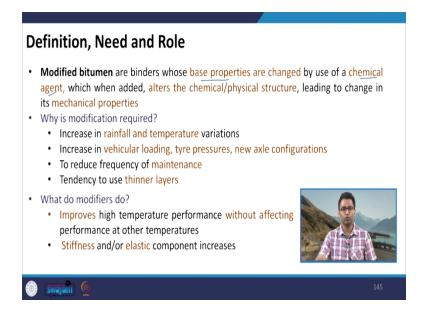
So, let us first see, what do we mean by modified bitumen, how do we define a modified asphalt binder or a modified binder or a modified bitumen. And let us also see that what is the need of modification, why do we need to modify the conventional asphalt binder and what is the role of this modification process.
