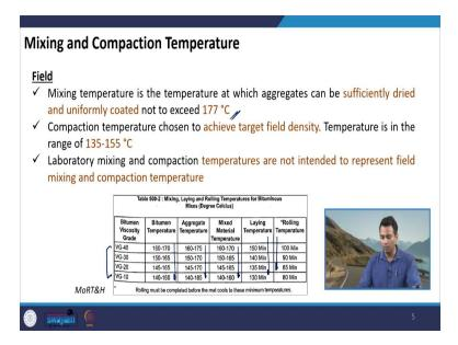
So, in the plant, how we determine the mixing temperature that at this temperature the aggregate can be sufficiently dried so, that we can remove all the moisture from the aggregates and then it can be uniformly coated with the aggregates and this temperature should not exceed 177 degrees Celsius as suggested by asphalt institute. Also, the idea for compaction temperature is to achieve the target field density and this this range can be between 135 to 155 degrees Celsius.
