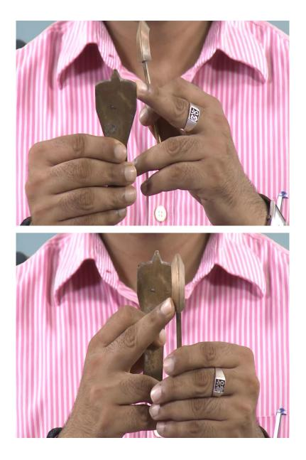
Again in my hand now, you can see both the tools. So, this is the Casagrande cutting tool, you can see this and this is the ASTM cutting tool. So, in this particular class I will be explaining the test using the Casagrande cutting tool, but you can use any of the cutting tools.
