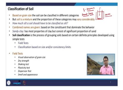
We have discussed that based on the grain size how the soil can be defined as a granular material as sand we have as coarse grained material, we have discussed about the sizes of sand, we know that what are the size range for silt, we also know what is the size range for clay. So, this is based on the grain size distribution.
