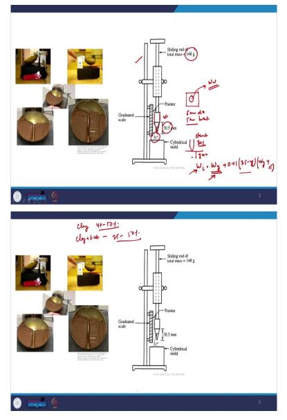
Another method which is again a popular method for determination of liquid limit is the use of a cone penetrometer which you can see here. So, what we do here again this is a simple experiment we have a cup, this cup has a specific dimension of, the dia is 5 centimetre and the height is again 5 centimetre. So, we will take the soil mass will mix it with water to make a paste and we will press it in this particular mould.
