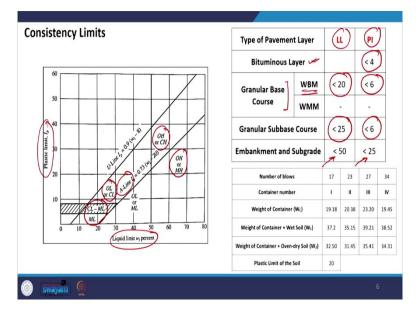
For example, this graph is typically used in the classification system. So, this is the graph from the unified soil classification system where we have A-Line. So, what A Casagrande did he studied different types of soil. And he plotted a relationship between plastic limit and liquid limit and depending on where the values lie, he divided this chart into different parts and where and which can be used to classify the soil.
