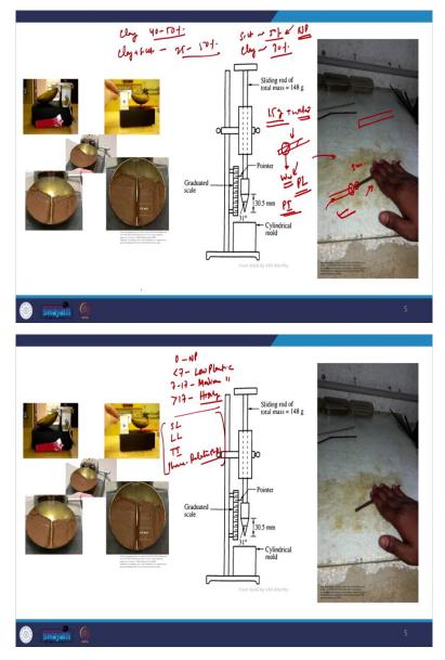
Let us now discuss about the plastic limit test again this is a very simple test, which you can do in the laboratory. So, what we do here we take 15 grams of sample passing 425 microns, we add it with water to mould the soil sample we will add that much water. Then what we do we will using the forefingers and a glass plate here, we will start rolling the sample, we will first make a small ball and we will start rolling the sample.
