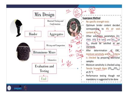
So, we are just completing so, I hope the previous explanation was clear how to do the complete the steps of Superpave Mix Design, coming to the Marshall mix design we have to plot the variations again here. But here in addition to the volumetrics, we are also looking at the stability and flow values which is plotted here.
