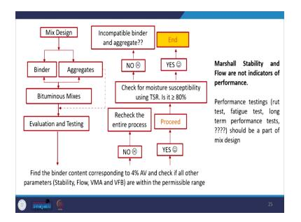
Coming to the Marshall Mix Design process as I said that, we will check all the other criteria's if these criteria's are not met then we have to recheck the design process. If it is met, then we will proceed, though usually not mandatory, but as per the guidelines of the ministry, we also perform a moisture susceptibility check using tensile strength ratio.
