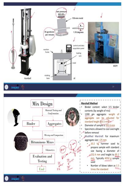
So, these are some images just to familiarize you with the different compaction process. So, this is a Marshall compactor you can see this is the compactor and this can be moved up and down this is the mold with the collar which I just showed you and using this machine we can produce the bituminous mixture.
