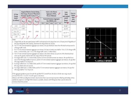
And this is the final criteria, which is outlined in the Superpave Mix Design method, which you can see that we have different criteria's corresponding to N initial, N design and N max and what should be the percent Gmm values. And then we also have criteria's corresponding to volumetric which we have already discussed does to binder ratio.
