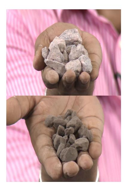
So, when I say hot recycle mixtures, I am basically talking about something which is popularly termed as RAP. So, RAP stands for reclaimed asphalt pavement. And what do we mean by reclaimed asphalt pavement it is not basically a pavement type as the name might indicate, it says reclaimed asphalt pavement but actually it is not a type of pavement rather it refers to removed or and reprocessed pavement materials containing asphalt and aggregates.
