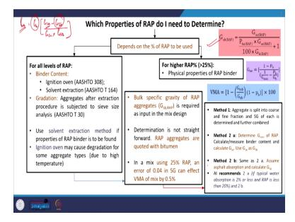
So, which properties of RAP do I need to determine? Well, this depends on the percentage of RAP I am intending to use in the final project or the in the final mix, irrespective of any percentage we use these properties we have to determine irrespective of any percentage ranging from more than 0 to let us say even 100 percent RAP you are targeting.
