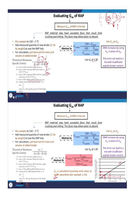
Now, when I said in method 2a, that you have to determine the Gmm of the RAP and using the Gmm and percentage, residual bitumen, we can calculate the Gse of RAP. The determination of Gmm of RAP is also not very, very straightforward, like the conventional method which we use for hot mix asphalt, well, the method remains the same, but some additional steps needs to be performed.
