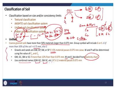
Let us try to understand step by step that how the unified soil classification system works. In this first you have to categorize the soil as either coarse grained soil, as fine grained soil, which means if I have a soil
