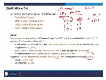
Now, let us go to the next step or the next domain that let us say that I took the soil I saved it through 75 micron and I found that more than 50 percent passes 75 micron which means that this soil now does not fall under the category of coarse grained soil that is gravel or sand no which means that this soil will now be classified using the primary classification will be either as silt or as clay or as organic silt or clay.
