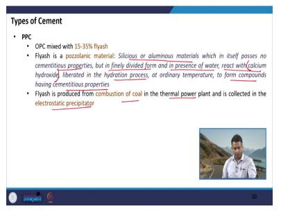
Let us talk about PPC which is a type of blended cement here what we do we mix OPC we have ordinary portland cement which is mixed with around 15 to 35 percent flyash. So, what is flyash, flyash is a pozzolanic material and how do we define pozzolanic material. So, pozzolanic materials are those or are basically Silicious or aluminous materials, which in itself posses no cementitious properties, which means,
