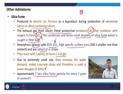
So, now, let us also discuss about few other mineral admixtures that are also used in the production of concrete. So, we have silica fume. So, how do we get silica fume silica fume is typically produced in electric arc furnace, which is as a byproduct during the production of elemental silicon or alloy containing silicon. So, during the production of silicon or alloy containing silicon in the electric arc furnace slag, we get a byproduct which is nothing but silica fume.
