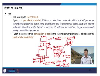
So, let us now see that what typically happens in the thermal power plant and as we all know that thermal power plant is meant to produce electricity and this happens using steam and then turning turbines.
