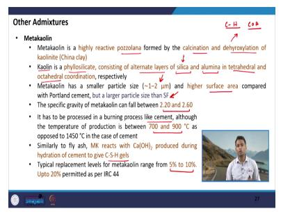
So, let us discuss about metakaolin now, again this is one of the products that is popularly being used in the production of concrete because of some of the unique benefits of this product. So, what is metakaolin it is a highly reactive pozzolana and we get metakaolin by calcination and hydroxylation of kaolinite.
