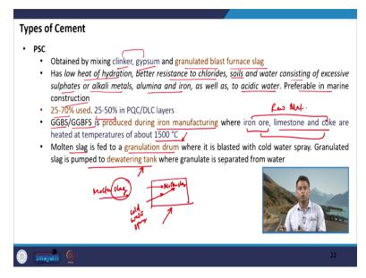
So, next type of cement that is Portland slag cement, Portland slag cement, it is obtained by mixing the clinker which we have during the production of cement gypsum which ultimately means that it is the Portland cement with granulated blast furnace slag.
