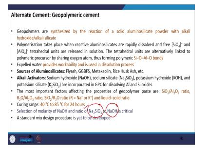
So, geopolymers they are synthetic synthesized by the reaction of solid aluminum silicate powder with alkali hydroxide or alkali silicate. So, this alkali silicate can be sodium silicate sodium hydroxide or it can be a potassium hydroxide potassium silicate. Now, polymerization it will take place when reactive aluminosilicates they get rapidly dissolved. So, we have to separate this alumina silicate bond.
