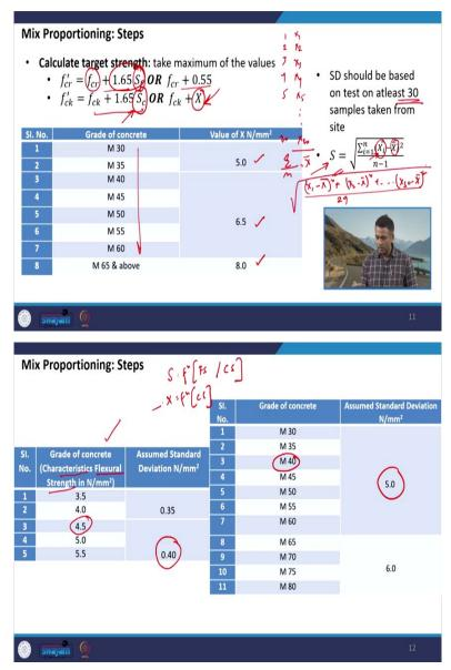
Or we can do the mix design also corresponding to the target flexural strength. So, usually when we see the concrete pavement design the critical failure mode of concrete is corresponding to the flexural stresses. So, flexural strength is considered as one of the design parameters to do the cumulative fatigue damage calculation. Therefore, it is also important that we should be able to do the mix design corresponding to the target flexural strength.
