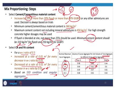
So, the next step now is to select the cement or the cementitious material content when I say cementitious material, it means that it can include a combination of cement and flyash or combination of cement and other mineral admixtures. So, that is why we call it either cement or cementitious material. So, how do we
