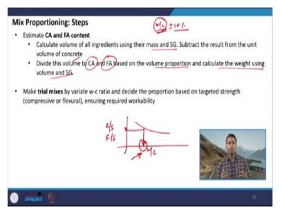
To finalize the proportions in terms of kgs per meter cube. So, calculate volume of all ingredients using their mass and specific gravity subtract the result from the unit volume of concrete, divide this volume to coarse aggregate and fine aggregate based on the volume proportion as we saw in the last slide and calculate the weight by using the volume and specific gravity. So, this will complete proportioning of different materials that we are going to use.
