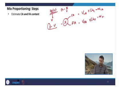
So, if you see the steps which we have talked about the water content, the cement content the admixtures they are all in terms of kgs per meter cube. So, usually we do the mix design of concrete considering a unit volume of 1 meter cube. So, and we have discussed about the proportions of materials in terms of kgs per meter cube.
