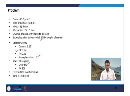
The type of cement which has been given to us is OPC 43. The nominal maximum aggregate size of the aggregate gradation is 31.5 mm, the workability has been defined as  $25 \pm 5$  mm, the average workability is 25 mm here, which we have to achieve. The aggregates that are being used to produce the mix are crushed angular aggregates.
