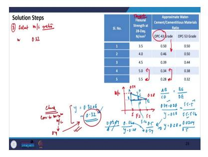
Now, let us move to the third step and the third step is to select the water cement ratio. So, in the third step we will be selecting water cement ratio. Water cement ratio is a function of the target flexural strength please remember that this is target flexural strength and the grade of cement. So, we have to look in this column because we are using OPC 43 here, our target strength was 5.16 which is somewhere between these two values. So, we have to interpolate accordingly.
