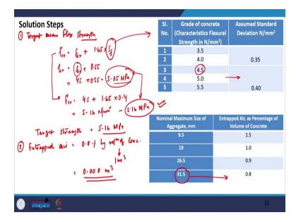
So, the first step as we discussed yesterday is that we have to calculate the target mean flexural strength so, we have to calculate the target mean flexural strength. So, if you remember that there were two equations corresponding to the flexural strength, one was that the value of f'cr = f cr which is  $F_{cr}$  +  $1.65 \times S_f$  and the second equation was that f'cr should be equal to  $F_{cr}$  + 0.55.
