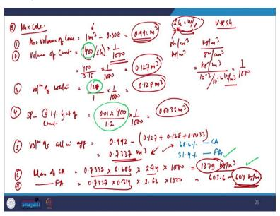
So, we will move to the next step that is the eighth step that is the calculation mix calculations. So, in the mix calculation coming to the first one, let us see the absolute volume of concrete it is  $1 \text{ m}^3$ , this is what we considered. But if we remove the amount of entrapped here this will be 0.008 as we calculated. So, this becomes equal to 0.992 m<sup>3</sup>.
