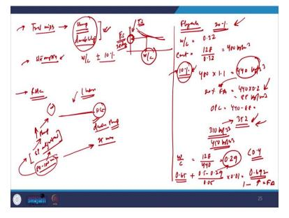
So, now, we have to make trial mixes. In the trial mixes for the calculated proportion, you check the slump requirement again and you also check for any durability criteria if there is any. Once these two criteria's are satisfied for the given proportion, then we will further check for strength. If let us say the initial proportion which you got that does not give you the required slump or durability some adjustments need to be made and accordingly the values will change.
