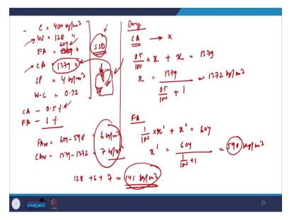
So, now finally, the proportions are let cement is equal to 400 kg/m<sup>3</sup> water is equal to 128 kg/m<sup>3</sup>, fine aggregate is equal to 604 kg/m<sup>3</sup>, coarse aggregate is kg/m<sup>3</sup>, superplasticizer is 4 kg/m<sup>3</sup> and then water cement ratio which wType equation here have taken is 0.32. But this is in an SSD condition.
