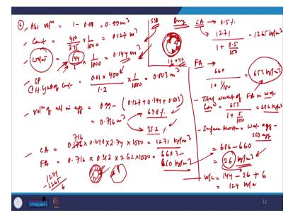
And then finally, we will have the proportions with us. So, let me write down the proportion. Now, in this problem the absolute volume of concrete becomes equal to (1-0.01). So, this is 0.99 m<sup>3</sup>. Then we have cement, we know the specific gravity, we know the mass, so we can calculate the volume which will be equal to 0.127.
