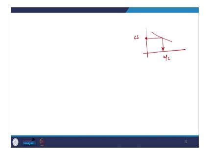
And then we will plot the graph between water cement ratio and the compressive strength or the compressive strength of the concrete. We will draw the graph, we know what is the target strength corresponding to the target strength what is the design water cement ratio we will estimate the same alright and this completes the mix design process as well. We will stop here today and we have discussed or we have solved a problem which is related to the mix design of PQC based on compressive strength.
