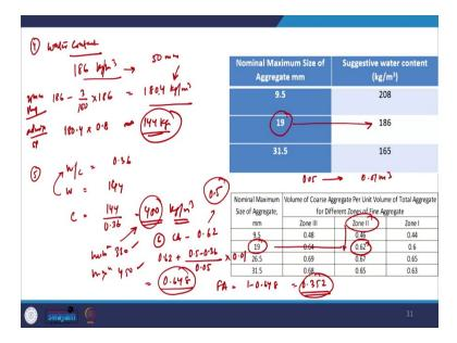
Again, we have a suggestive table corresponding to the NMAS. So, the nominal maximum aggregate size is 19. So, the suggestive water content is  $186 \text{ Kg/m}^3$ , but this has some conditions. For example, this is for a slump of 50 mm. And this is without any admixture. So, similar to what we did in the last problem, our design slump is 25. So, we have to reduce 3 percent.
