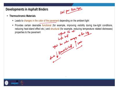
Another interesting material that can be used are thermochromic materials. So, these materials will change the color of the pavement depending on the ambient light. So, these are materials that have higher reflectivity as well as emissivity to solar radiation. Now, other than thermochromic materials, there are other materials as well, that has high reflectivity.
