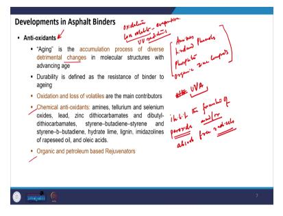
Then, we also have antioxidants. So, antioxidants are basically materials that helps us to improve the resistance of bitumen towards aging and we have already discussed in detail about the aging phenomena, which is the accumulation process of diverse detrimental changes. And these changes are built in because of probably oxidation, loss of volatiles.
