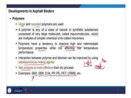
So, if you talk about the development in asphalt binders, various technologies can be listed. For example, use of polymers, we have already discussed about polymer modified binder what are they, but, these polymers in different forms are being developed and are being used at varying dosages to improve the rheological response, to improve the mechanical response of asphalt mixtures. Polymers are being used both in virgin and in recycled form.
