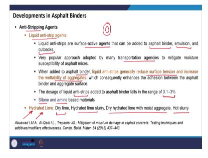
We also have anti stripping agents. So, this is used to resist moisture damage in the asphalt mixtures. Again anti stripping agents can be of different types. We have commonly liquid anti stripping agents are used. So, this liquid anti strip agents they are surface active agents that can be added directly to the asphalt binder, it can be added to emulsion or it can also be added to cut backs if we are talking about cold bituminous mixture as well.
