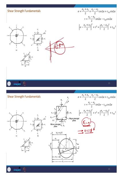
If you talk about the Mohr coulomb failure theory, if  $\sigma_1$  and  $\sigma_3$ . Now, see the Mohr coulomb envelope, so, this will be the plane of failure. So, this will be equal to  $\frac{\varphi}{2} + 45$  and now, using this also we can try to understand the Mohr coulomb failure envelope so, we know the orientation of this plane now.
