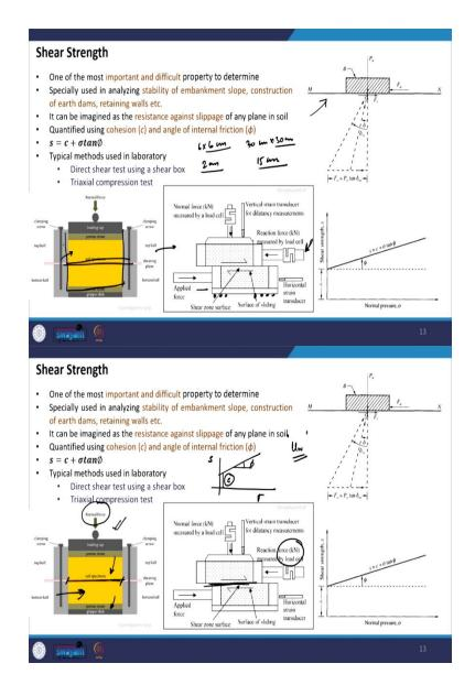
This is what we have discussed. Now, the next question is that, how can we evaluate the value of these shear strength parameters in the laboratory? So, there are two popular methods that are typically used one is the direct shear test using a shear box and the other is a tri-axial test, let us learn about these methods, we will start discussing about the direct shear test using the shear box.
