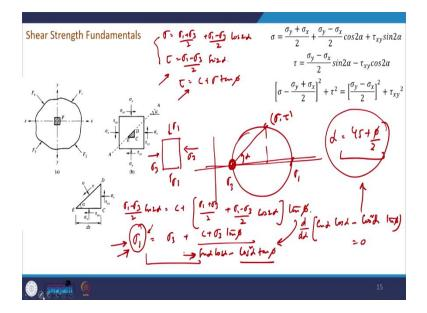
So, if you try to draw the Mohr circle, so, the Mohr circle will be a similar circle, but here this will be equal to  $\sigma_3$  this will be equal to  $\sigma_1$  and where is the pole the pole is actually these points the, because we know the value of  $\sigma_3$  and  $\sigma_1$  and  $\tau$  is equal to 0 so, it will coincide with the x-axis.
