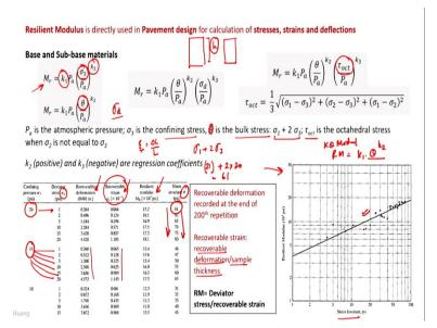
So, as I mentioned resilient modulus is directly used in the pavement design for the calculation of stresses, strains and deflection. And that is why we are interested to find out the resilient modulus. Usually, for base and sub-base material, so, if you see the soil for cohesive material, the response is typically different then what we will expect for a cohesionless soil or granular soil.
