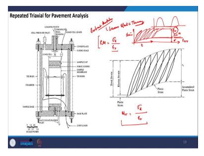
Similarly, in for soil that is the subgrade material also we use the triaxial test, but not specifically to assess the value of c and phi, rather, we perform a repeated triaxial test to get the permanent strain in the
