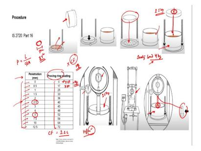
I will first locate the point from where this straight part starts and I will make a tangent. So, I will make a tangent here and I will mark this point. So, this will be the New (0, 0) point which means I have to shift the axis from here to here, likewise all the values will be shifted to equal amount, I mean to equal distance. I am interested in let us say 2.5 mm penetration.
