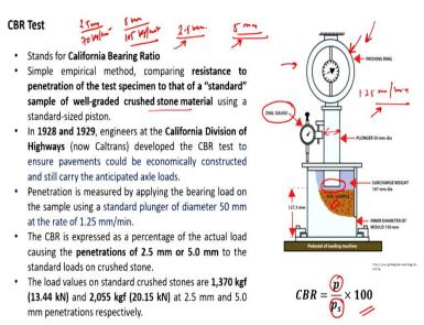
You can see that how the machine looks like. So, this is just a pictorial view of the CBR testing machine here. The value which we get using this test method that is the California bearing ratio is empirical in nature and it is used for comparing the resistance of penetration to the test specimen with a standard sample of well-graded crush stone material.
