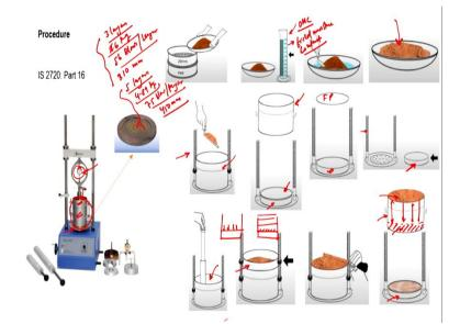
Now, let us look at the test method we will talk about the test method. Now, so, the Indian Standard code for this test method is IS2720 Part 16. This picture shows an example of the CBR testing machine which you can see that this is the proving ring here as I showed you in the last slide.
