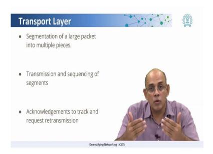
So, the function of the network layer is very similar to the function of the postal system when you are sending one letter. Going ahead you might have more than one letter, you might have large packages which have to be sent, such as we saw in the analogy example. So, in this case what is required is that, you want to take a large document and you want to chunk it into multiple pieces, you want to segment it into multiple pieces and send each of them through the network layer.
