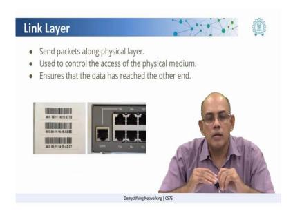
On top of the physical layer is, what we call the link layer. So, what is the link layer? The link layer now has to concern itself with transmitting what are called packets or segments along the physical layer. For example, let us say you are using a wireless network, it may be that there
