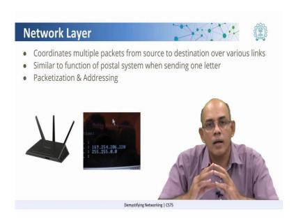
What comes above the link layer? It cannot be that everything is just one link. So, automatically we need the notion of being able to have multiple links which are connected with each other in order to form a network. The moment we do that we automatically come up with the idea of packets, saying that I need a packet, now this packet has to go from a source which is at one end of the network to a destination which is at another end of the network and in between there could be multiple links.
