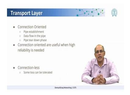
One is called a connection orientated protocol in which case basically there is a connection between the sender and the receiver. You can imagine the connection as a pipe where first there is the pipe establishment phase, then there is data which flows along the pipe and then there is a pipe tear down phase ok. This connection oriented protocols are useful when we want highly reliable communication in which the loss is cannot be tolerated by the system.
