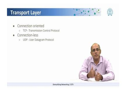
The examples of these protocols are, in the case of connection oriented we have TCP which is called Transmission Control Protocol and in the case of connection less we have UDP which is called User Datagram Protocol.
