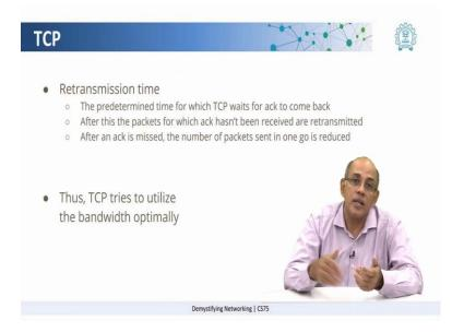
That again is a new concept which is called the retransmission time out. So, at this point we can just think of it as a predetermined time that TCP waits for the acknowledgement to come back. If the acknowledgement does not come back in time, then once again it starts, it drops the values and it starts again from a smaller value of number of packets to be sent.
