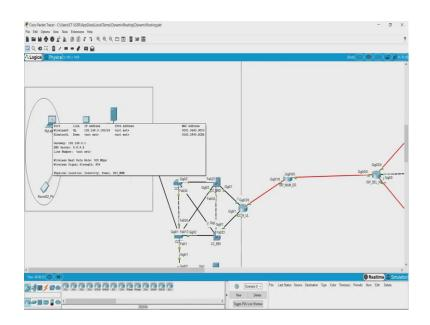
I am working with the same network that you are familiar with. One of the useful command is the ping command where you can ping any logical address or any IP address and see that whether the device with that address is reachable from your system or not.
