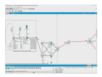
If you look at this router, it has 192 series address for the LAN network and both of these devices should have IP addresses belonging to, IP address belonging to 192 series. If you are statically assigning IP address,
