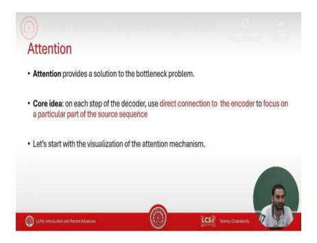
So this is the philosophy of attention I already mentioned about this bottleneck problem right So what is attention? The core idea here is that on each step of the decoder We use a direct connection to the encoder to focus on a particular part of the source sequence.
