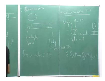
So, think of a configuration of a Turing machine. So, what do have in a configuration of a Turing machine? If you look at the configuration of a Turing machine, It has 3 things. It has a current state; it has the current tape contents and it has the position of the tape head. We have a state q and in the tape basically I am pointing to a particular cell. If you have a deterministic Turing machine, the transition of a deterministic Turing machine is as follows.
