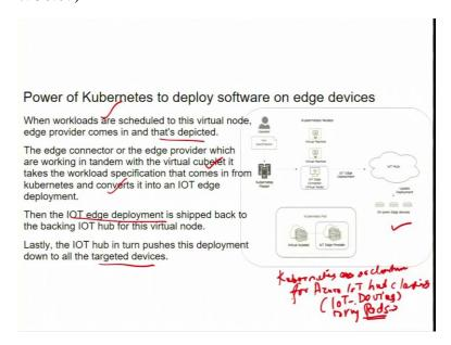
So, when a workload are scheduled to this virtual node edge provider comes in, that is depicted over here. So, the edge connector or the edge provider which are working in tandem with the virtual kubelet it takes the workload specification that comes in from the kubernetes and converts it into an IOT edge deployment. Then this IOT edge deployment is shipped back to the backing of IOT hub for it is virtual node.
