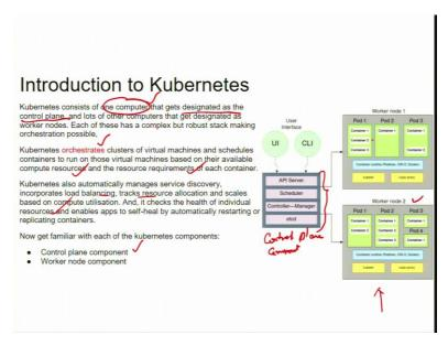
So, the Kubernetes consists of one computer that gets designated as a control plane. When we say computer may not be the physical computer, it may be the virtual machine as well. So, this particular Kubernetes has a designated system and that is called a control plane. Now, each of these has the complex, but robust stack making this orchestration possible.
