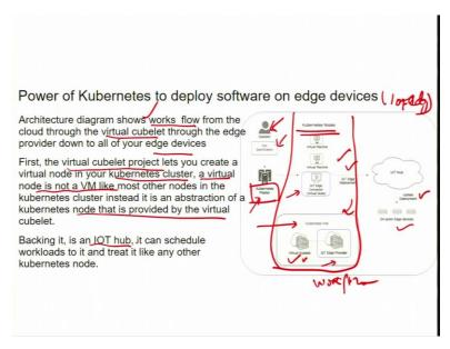
Now, let us see that how kubernetes you can use to deploy the software on the edge devices. So, this also is applicable for an IOT edge. So, the architecture shows the flow from the cloud through a virtual cubelet. So, here you can see this particular illustration the workflow from the cloud through the virtual cubelets through the edge provider down to your edge devices.
