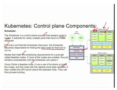
Now, comes finally, the last component in the control plane called scheduler. So, scheduler is the control plane process that assigns parts to the nodes. So, when we say node we mean that the worker node and this becomes the cluster, Kubernetes cluster, part of the Kubernetes cluster. So, the unit of assignment is called the pods and the pods contains the cluster. So, therefore, the scheduler is a process that assigns pods to the nodes.
