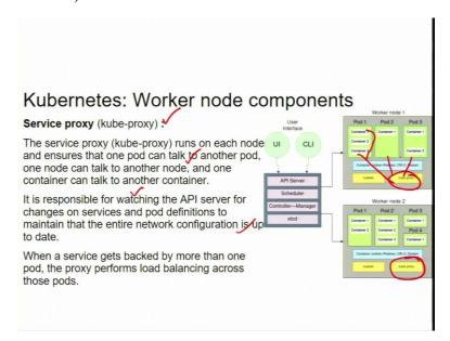
Then comes the kube proxy. The kube proxy also runs as a service in every node, worker node. So, the kube proxy runs on each node and ensures that one pod can talk to another pod and one node can talk to another node and one container can talk to another container. So, that means, kube proxy becomes a point of interaction or a communication just like you can think of a proxy server working in the internet for internet connectivity.
