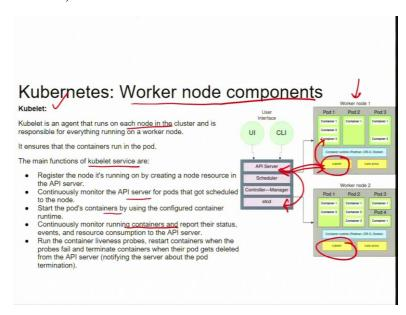
Finally, now we will be looking up the worker node components. So, in the worker node if you see there is a component which is called a kubelet. So, kubelet is an agent that runs in each node you can see that here there is an example of two nodes - in every node this kubelet is running as an agent responsible for everything running on the worker node.
