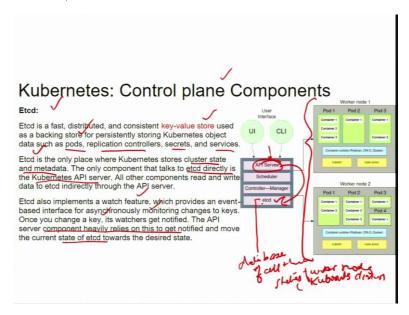
So, Kubernetes control plane components comprises of Etcd. So, Etcd that is Etcd daemon also is a fast distributed and consistent key value store, used as the backing store for persistently storing Kubernetes object data such as parts, replication, controllers, secrets and services. Therefore, this Etcd is a database of all the states information of the worker nodes, that is the Kubernetes cluster.
