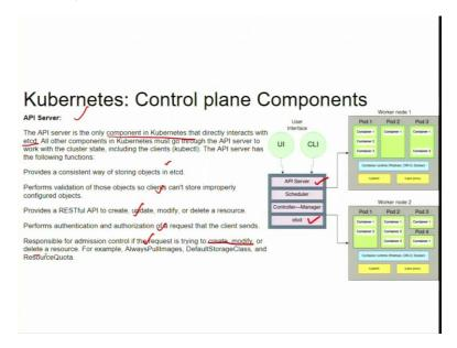
The other component of a control plane is API server. API server is the only component in the Kubernetes directly interacts with Etcd that we have already seen in the previous slide. So, the API server has the following functions. The first one is it provides the consistent way of storing the objects in Etcd, it performs the validation of these objects.
