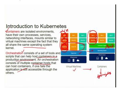
So, introduction to Kubernetes. Let us introduce two concepts to understand the background for Kubernetes. So, the containers is an isolated environment to have their own process, services, networking interface for an application that mount similar to the virtual machine except the fact that they all share the same operating system kernel.
