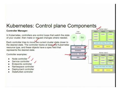
Now, we will look to the controller manager that is the third component of the control plane. So, in Kubernetes controllers are the control loop that watch the state of your cluster and then make the request changes wherever it is needed. Each controller tries to move the current cluster state closer to the desired state.
