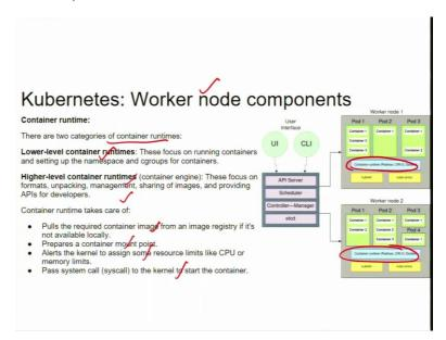
Similarly, now there is a thing which is called a container runtime. So, container runtime is also a worker node component. So, it has two categories of container runtime - one is that lower level container runtime focuses on running containers and setting up the name space; a high level container runtime focus on formats unpacking management and sharing of the images.
