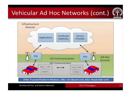
So, here is a diagram of the overall order of vehicular Ad Hoc networks. So, as we can see that, we have vehicles in one layer and each of these vehicles as you can see have the electronic circuitry the OBU then the trusted you know module which is known as the trusted platform module TPU. You know that for module and the vehicles also have different sensors which collect different information from the vehicle from you know the behavior of the driver and so on and so forth.
