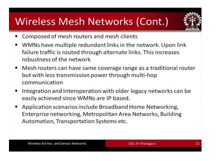
So, as you as I told you that, we have mesh routers and mesh clients typically, these mesh routers they would be configured in a you know in a mesh like configuration which helps in improving the reliability of the networks and reliability of communication between the different nodes in the network they also have different types of application scenarios, broadband, home networking enterprise networking, metropolitan area networking, building automation transportation and so on and so forth.
