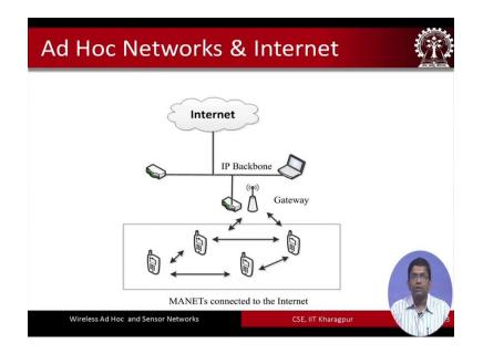
Here is an example of Ad Hoc networks is connected to the internet. Ad Hoc networks may or may not be connected to the internet this is an example of Ad Hoc network which is connected via an IP backbone to the internet.
