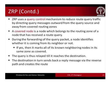
So, ZRP uses a control very control mechanism to reduce the route query traffic by directing query messages outward from the query source and away from the covered routing zones. Basically, there is a concept of a node being covered. A covered node is a node which belongs to the routing zone of a node that has received a route query.
