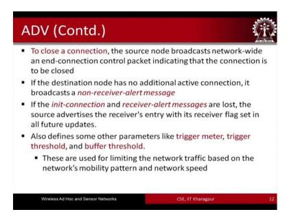
Now, to close the connection the source node broadcasts the network quite end connection control packet indicating that the connection is to be closed. So, end connection is the control packet that is used and broadcasted by the source node to the entire network when it is required to terminate a connection. If the destination node has no additional active connection it broadcasts a non-receiver-alert message; again a type of message that is proposed in this particular protocol the ADV protocol.
