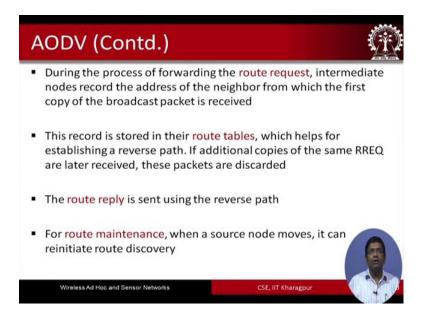
So, during the process of forwarding the route request intermediate nodes record the address of the neighbor from which the first copy of the broadcast packet is received. This record is stored in the routing tables, which helps for establishing a reverse path. If additional copies of the same RREQ are later received these packets are discarded. So, this is very interesting actually I will highlight this once more later on. So, basically you know here the help of routing tables is taken.
