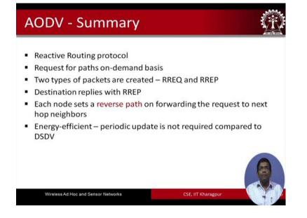
In some it is a reactive routing protocol, which requests for paths on demand. Two types of packets are used: RREP and r r e sorry; RREQ and RREP. The destination replies with RREP corresponding to the RREQ that it has received from the source file all the intermediate nodes. And each node sets a reverse path on forwarding the request to the next hop neighbors. This is more energy efficient where periodic update is not required compared to DSDV.
