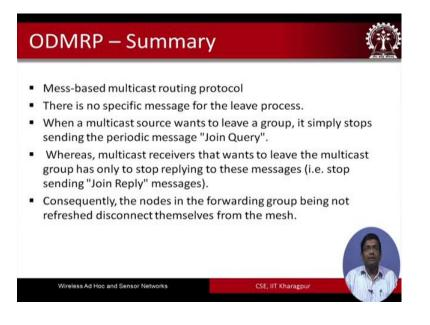
So, mesh based multicast routing is adopted. So, there is a small type way. So, it is m e s h not m e s s. There is no specific message for the (Refer Time: 25:53) process when a multicast source wants to leave a group it simply stops sending the query message whereas, multicast receivers that want to leave the multicast group has to stop sending the reply message. Consequently the nodes in the forwarding group being not refreshed will disconnect themselves from the mesh.
