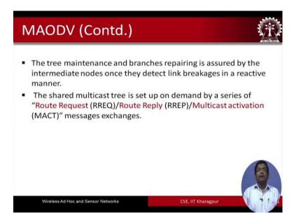
The tree maintenance and branches repairing is assured by the intermediate nodes once they detect link breakages in a reactive manner the shared multicast tree is set up on demand by a series of RREQ route requests, RREP route reply and MACT multicast activation message exchanges.
