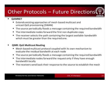
So, now we are not going to go through any of the other multicast routing protocols in further detail, but I would just like to mention that there are many others few of them are given over here. QAMNET is a multicast routing protocol; QMR is another multicast routing protocol which basically is based on quality of service guarantees. So, QoS multicast routing protocol is the full form of QMR.
