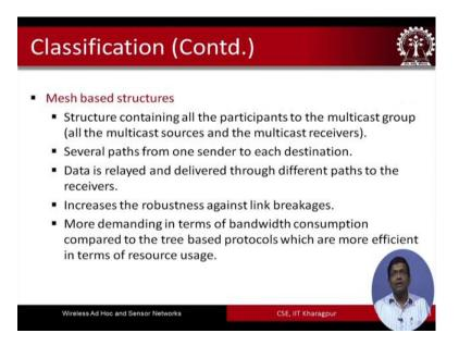
Mesh based structures I do not need to elaborate any further it is a mesh based structure that is adopted we are increasing the redundancy means we are increasing reliability, but we are also increasing at the same time the overhead because the same packet is going to flow around through a multiple links from multiple possible links from the source node from which the packet is going to MANET. (Refer Slide Time: 20:20)
