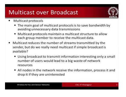
The main goal of multicast protocols is to save bandwidth by avoiding unnecessary data transmissions multicast protocols maintain a multicast structure to allow each group
