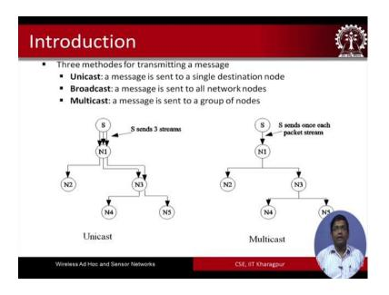
So, let us look at these figures. So, there are 3 methods for transmitting a packet - one is unicast that means, a message is sent to a single destination node as we can see in this particular figure. So, here as we can see that this is from S 1 to N 1 there is one stream from S 1 to N 2 there is another stream S 1 through N 3 another one and so on. So, this is an example of unicasting.
