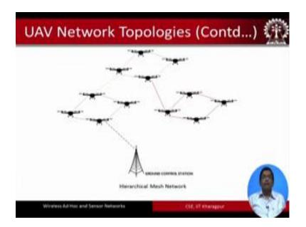
So, this is how a flat mesh network looks like. So, here what we have is a hierarchical mesh network and this is quite obvious. So, not only that we have a flat mesh like configuration, but from here again there it basically connects with another mesh and from this mesh again there is connectivity to another mesh. So, this is how different hierarchies are formed. And we have a hierarchical mesh network and from this mesh network there is connectivity to the ground control station
