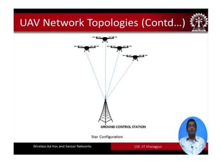
So, this is the star configuration as we can see that this is the star topology. So, these are the UAVs the 4 UAVs they connect with the ground control station. And this is how the star topology looks like here.
