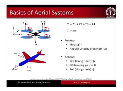
Some of the basics of any aerial system and particularly in the context of UAVs. So UAV is a flying device an unmanned flying device. So, the way a UAV flies is because of a thrust because of the thrust. So, let us say that we have we have an UAV like this. So, this UAV has 4 different propellers and so the different forces that are acting on this UAV are as shown.
