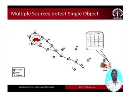
Now, we have the scenario of multiple sources multiple sources detecting a single object. So, we have nodes 1 2 4 15 and17 these blue colored nodes which have all together sensed the presence of a vehicle.
