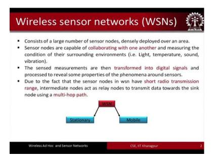
So, as I told you that a wireless sensor network basically consists of a collection of different sensor nodes. And these sensor nodes are typically not necessarily, but typically they are densely deployed in an area. So, the sensor nodes they basically communicate with one another the sensor nodes first of all they have the capability of sensing the physical phenomena that are occurring around them. For example, the examples of whatever I told you already like for instance.
