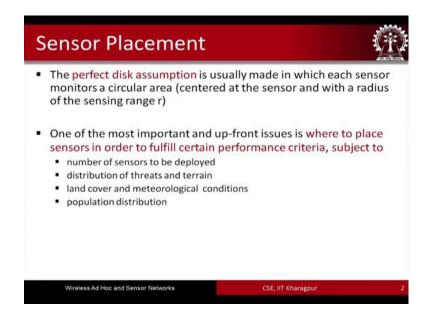
So, first of all in the sensor placement problem, it is assumed that there is a perfect disk that is used for deployment and that perfect disk assumption is usually made in which each sensor monitors a circular area that is centered at the sensor and with a radius of the sensing range r and this particular thing when we this particular concept we had covered in the previous part of this topic as well there I spoke about the not only the disks, but also the concept of unit disks.
