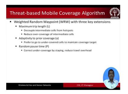
So, there is a an algorithm the WRP algorithm which is which is a thread based mobile coverage algorithm that is proposed and I am not going to go through it in detail, but just to give you a little bit of feeling of what it does. So, 3 different parameters are considered one is the maximum trip length the second one is the adaptivity to prior coverage and the third one is the random pause time. So, 3 different criteria are considered and a mobile coverage algorithm is proposed.
