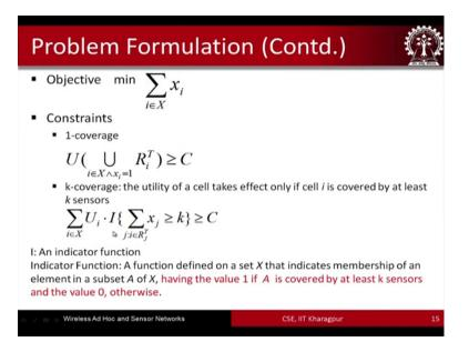
The objective function is to minimize the summation of all these X is and there are 2 constants if it if we are talking about the one coverage problem the constraint is like this that utility of the union of all these arise that should be greater than or equal to C which is the coverage requirement and if it is a K coverage problem the corresponding constraint equation is as shown.
