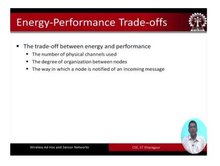
There are different tradeoffs between energy and performance with respect to the number of physical channels used, the degree of organization between the nodes and the way in which a node is notified of an incoming message.
