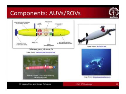
So, AUVs and ROVs autonomous underwater vehicles and remotely operated vehicles these are things which are also used in conjunction with UW essence. So, these are the pictures of autonomous underwater vehicles. So, these autonomous underwater vehicles can also act as data mules so which will collect the data from these different sensor nodes underwater sensor nodes and to being the data to a different point maybe surface of the surface of water or whatever.
