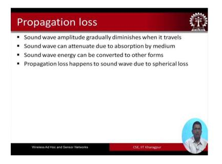
There is lot of propositions loss there is not a propagation loss the sound waves amplitude basically diminishes quite fast then the second thing is the sound waves gets attenuated due to absorption by the medium. Third is that the sound wave energy can be converted to other forms and the propagation loss happens to sound waves due to spherical loss.
