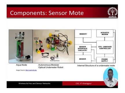
Now here is a on the on the left hand side what we see over see is basically and you know a pictorial view of underwater sensor node which is called the aqua node, a
