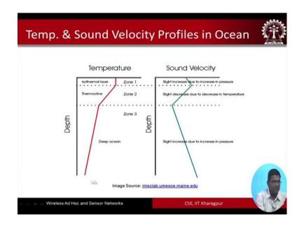
So, pictorially let us look at 2 of them one is the temperature variation with depth and the sound velocity variation. So, this is what we see; so, you when we talk about the oceanic column. So, it is basically typically it can be segmented into different layers or different zones. So, the first one is the isothermal layer then we have the thermo cline layer and then we have the deep ocean layer. So, these are the different zones.
