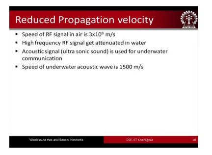
So, there are other properties of the signal velocity. So, for RF in here you know it is 3 into 10 to the power 8 meters per second the speed the high frequency RF signal gets eliminated in the water acoustic signal is used for underwater communication and the speed of underwater acoustic waves is 1.5 kilometers per second. So, 1500 meters per second this is the speed of underwater signals underwater wave acoustic waves.
